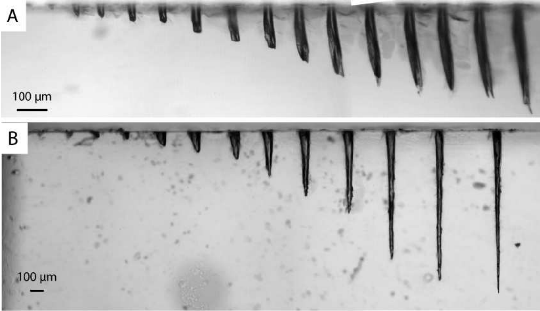
Figure 2: A. side view of an ablation serie from N=100 to N=3000 using the long focal lens. B. Side view from an ablation serie produced by the short focal objective (N=100 to N=3000)
