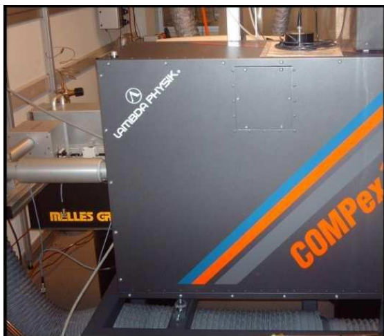
Figure II.12 : Laser Excimer type Complex (Lambda Physics).
