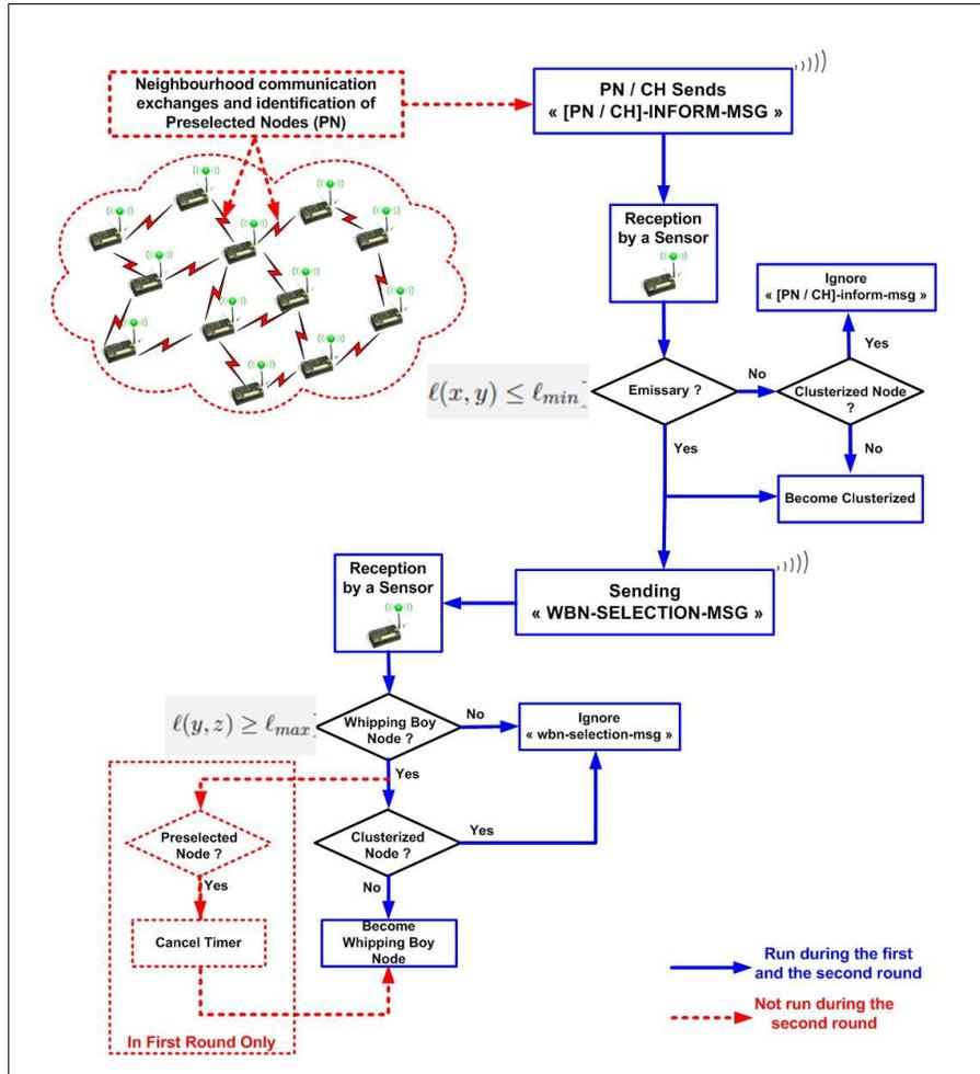
FIGURE 8.4: The LQI-DCP Protocol Flowchart : 1<sup>st</sup> and 2<sup>nd</sup> Round. Contrary to the « PN-INFORM-MSG », the « CH-INFORM-MSG » messages are firstly sent during the 2<sup>nd</sup> Round by the non clusterized nodes and then by the Whipping boy nodes.
