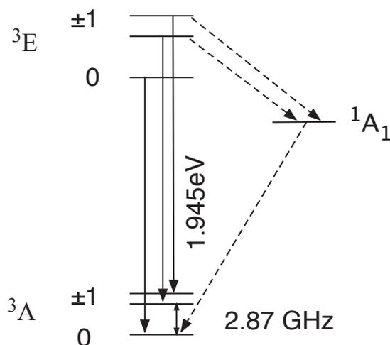
**Figure 5.2:** Schematic energy level structure of  $NV^-$  color center, the transition from the excited state ( ${}^3E$ ) to the ground state ( ${}^3A$ ) is spin preserving and produces broad band PL with ZPL at 637 nm,  ${}^1A_1$  is a dark state. The electron relaxation through this state is no radiation and non spin preservation. The ground state is a triplet. The zero field splitting between  $|0\rangle$  ground state and  $|\pm 1\rangle$  ground is 2.87 GHz.
