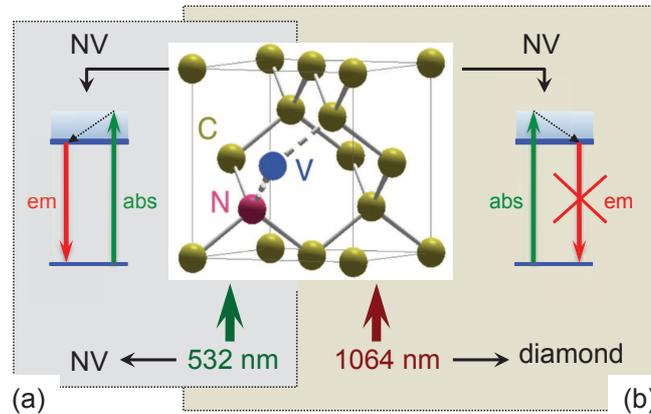
**Figure 3.13:** Proposed mechanism of the photoluminescence quenching effect of NV color centers due to the IR excitation. (a) NV color center in diamond crystal absorbs only 532 nm light and emits luminescence. (b) NV color center absorbs 532 nm light while diamond crystal absorbs 1064 nm via multi-photon absorption process. The later is shortly (during pulse duration) ionized and it affects (quenches) the photoluminescence of NV color center.
