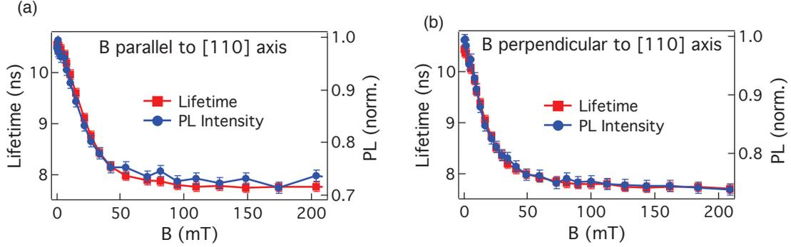
**Figure 7.4:** Measurement of PL intensity and PL lifetime as a function of  $\mathbf{B}$  magnitude. (a)  $\mathbf{B}$  is parallel to the [110] axis. (b)  $\mathbf{B}$  is perpendicular to the [110] axis. The PL intensity changes with a clear correlation with the lifetime modification, both of them decrease obviously with the magnetic field intensity.
