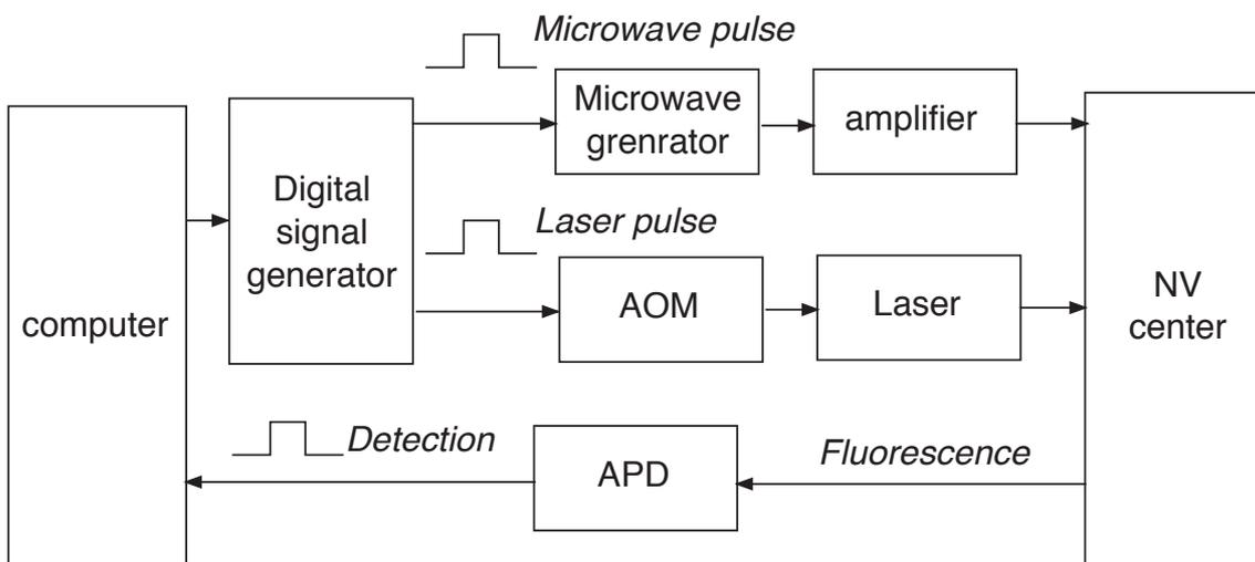
**Figure 5.5:** Pulsed ESR hardware scheme. The microwave generator is triggered by a digital signal generator interfaced with a computer, and the output is amplified by an amplifier. Laser is switched by AOM which is also triggered by the digital signal generator. The fluorescence is detected by the APD.
