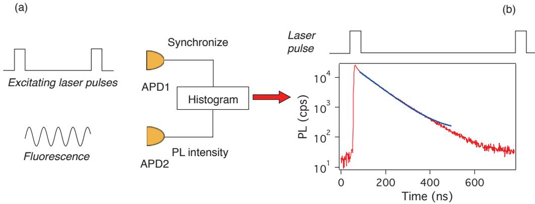
**Figure 5.7:** Lifetime measure of NV color center. The laser pulse is used to synchronize the data acquisition, the PL decays after the laser pulses. By fitting the PL decay curve exponentially, the decay rate is considered as the PL lifetime.
