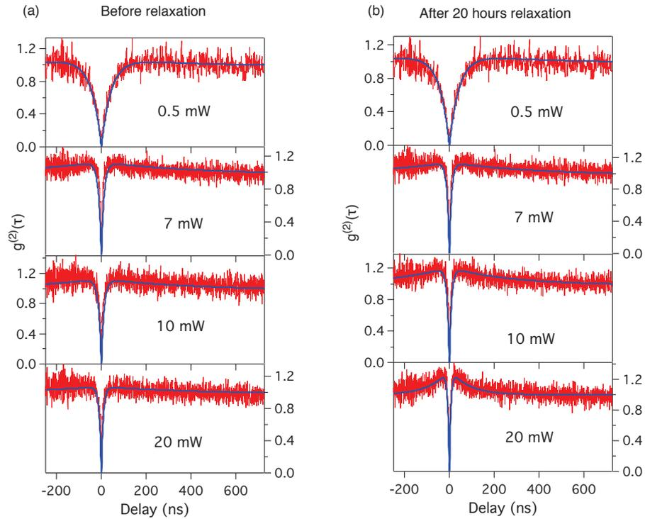
**Figure 2.12:** Relaxation of photochromic effect. Figures at left:  $g^{(2)}$  measurements of the NV center obtained just after a strong irradiation, the color center is ionized to a neutral charged state. Figures at right:  $g^{(2)}$  measurements of the same NV center obtained after 20 hours relaxation, the color center remains single,  $NV^0$  returns partially to  $NV^-$
