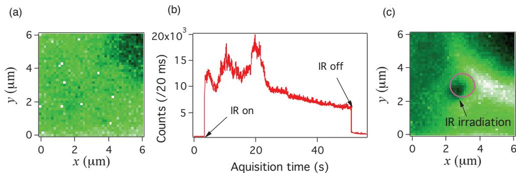
**Figure 3.11:** IR effect on the photoluminescence of NV color centers in a bulk diamond. The IR pulses burn the diamond surface at very low power (40 mW). The burning effect is immediate and no diminution of photoluminescence signal is observed. (a) and (c): scanning pictures obtained before and after 40 mW IR irradiation. (b) photoluminescence as a function of the acquisition time. The moments of turning on and off of the IR pulses are indicated.
