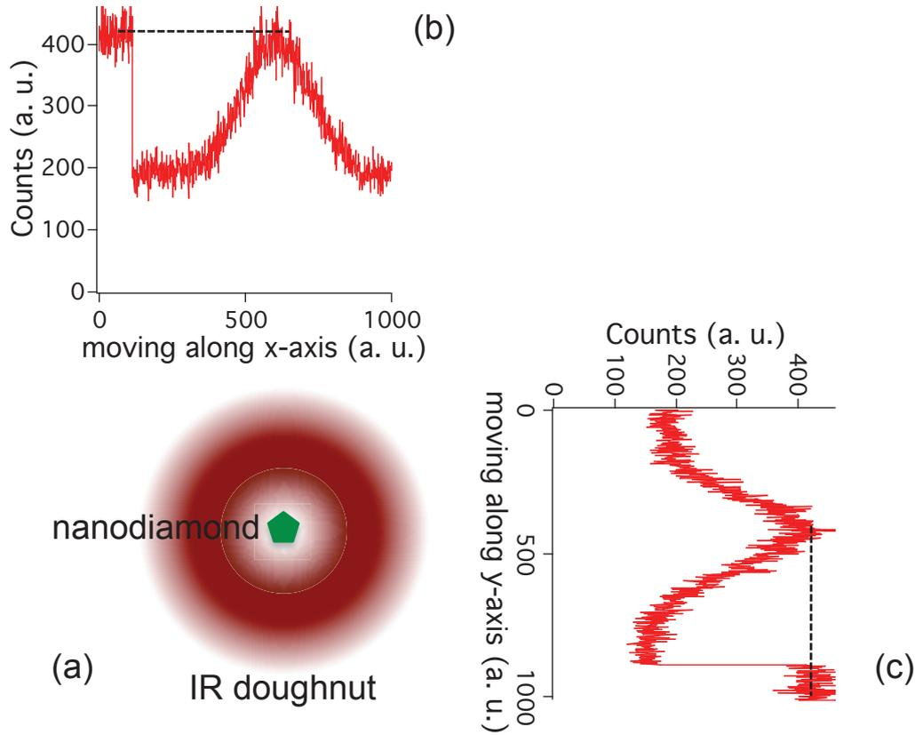
**Figure 4.8:** A luminescence nanodiamond is excited by a combination of an Airy green beam and a doughnut IR beam. (a) When the IR doughnut beam is well aligned with nanodiamond, there is no IR excitation and no thermal effect. When the nanodiamond is raster scanned by this combination, the photoluminescence is modulated as shown in (b) for the a moving in  $x$ -direction and in (c) for a moving in  $y$ -direction.
