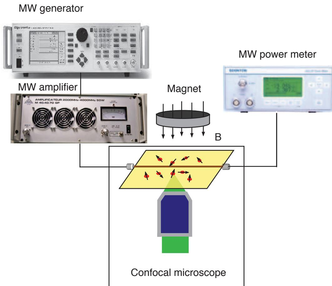
**Figure 5.4:** The setup for NV spin manipulation, the microwave is sent through a thin copper wire which is close to the sample surface. The magnetic field is applied with a magnet, the magnetic field can be controlled by moving the magnetic in 3D space.
