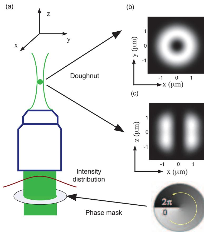
**Figure 4.6:** (a) A doughnut shaped focal spot is formed by using a  $2\pi$  phase modulating mask, Calculated intensity distribution of the focusing point in the transverse direction (b), and in the longitudinal direction (c).
