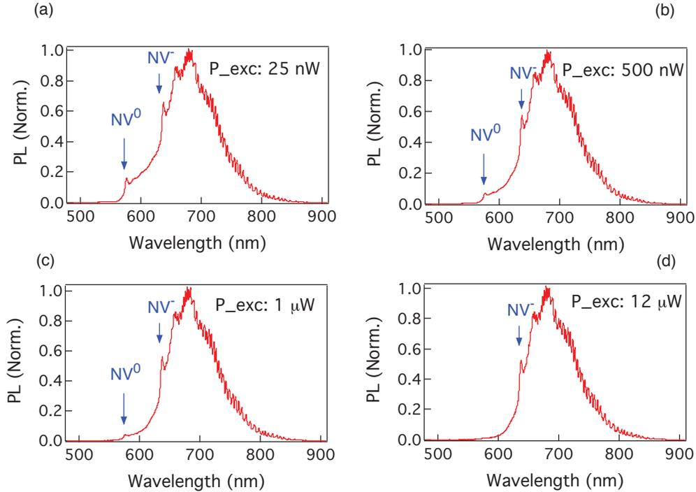
**Figure 2.9:** PL spectra of a proton irradiated HPHT bulk diamond taken at different excitation power, ZPL of  $NV^0$  decreases with excitation power and disappears at an excitation power stronger than  $8 \mu\text{W}$ . The sample contains multiple NV color centers and it is excited by a continuous laser at  $\lambda=532 \text{ nm}$ .
