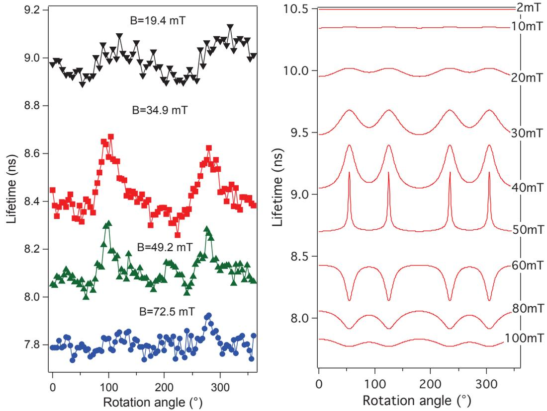
**Figure 7.5:** Lifetime measurement by rotating  $\mathbf{B}$ -orientation on the [110] plane. (a) Experimental result, the measurements of 4 different  $\mathbf{B}$  magnitudes (19.4 mT, 34.9 mT, 49.2mT and 72.5 mT) are made. (b) Calculation result of the ideal case: all the NVs including the density and orientations are uniformly distributed. Lifetime of  $|0\rangle$  and  $|\pm 1\rangle$  states are 10.5 ns and 7 ns respectively.
