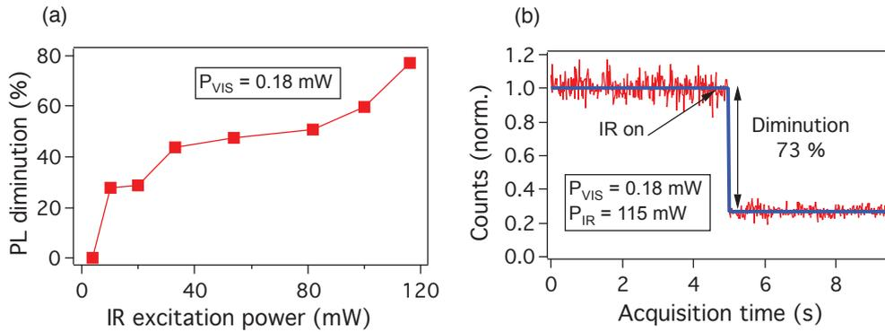
**Figure 3.8:** Photoluminescence quenching effect obtained by different IR excitation powers. (a) Normalized diminution of the luminescence as a function of IR power. (b) Photoluminescence as a function of time obtained without and with IR excitation, showing the best modulation.
