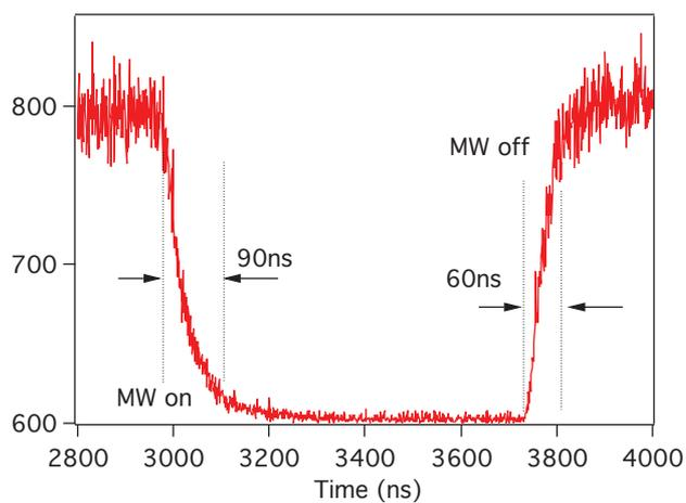
**Figure 5.6:** The instrument response time to the microwave signal. When the microwave signal is switched on the response time is about 90 ns, when the microwave signal is switched off the response time is about 60 ns.
