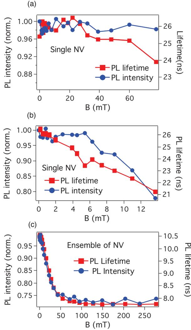
**Figure 6.6:** PL intensity and PL lifetime of as a function of  $\mathbf{B}$ -magnitude. (a) Measurement of single NV center when  $\mathbf{B}$  has small angle to the NV axis. (b) Measure of single NV center when  $\mathbf{B}$  has larger angle to the NV axis. (c) Measurement of an ensemble of NV center.
