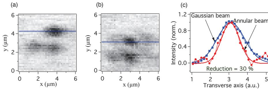
**Figure 4.5:** Super-resolution with an annular beam. Photoluminescence scanning image obtained with a gaussian beam (a) and with an annular beam (b). (c) Profile of the photoluminescence spot of a NV color center corresponding to the lines in (a) and (b).
