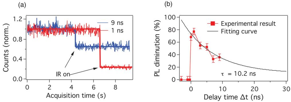
**Figure 3.5:** (a) Photoluminescence diminution obtained by  $\Delta t = 1$  ns and  $\Delta t = 9$  ns. (b) Photoluminescence quenching as a function of the time delay,  $\Delta t$ . The black curve is the monoexponential fit showing a time decay of the photoluminescence of about 10.2 ns, similar to the decay lifetime of the NV color center.
