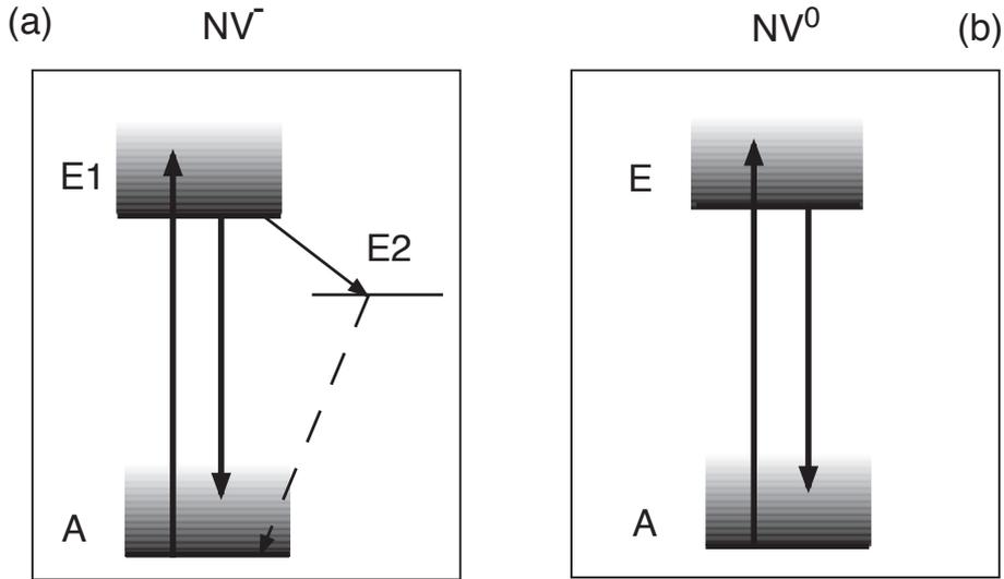
**Figure 2.7:** Proposal of energy diagram of  $NV^-$  and  $NV^0$  color centers. The 2-level structure of  $NV^0$  center allows obtaining a perfect antibunching curve, while the 3-level structure of  $NV^-$  color center causes the bunching effect.
