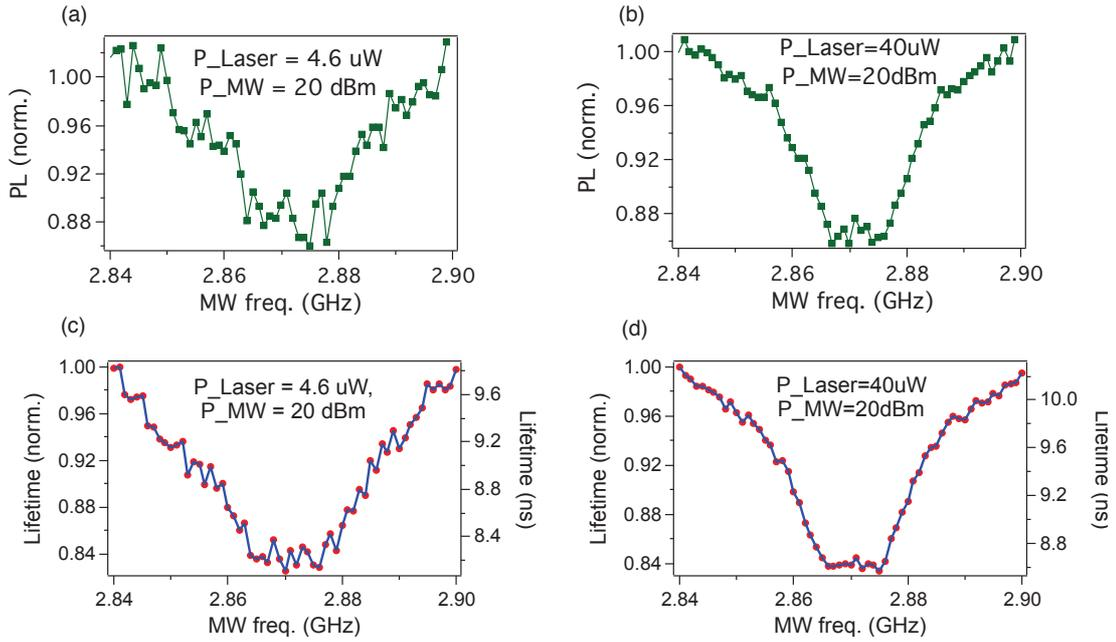
**Figure 6.5:** Measurement of PL intensity and PL lifetime of NV color by sweeping the microwave frequency around the ESR resonance frequency. (a) and (b) are PL intensity measurements with excitation laser power of  $4.6 \mu\text{W}$  and  $40 \mu\text{W}$  respectively. (c) and (d) are PL lifetime measurements with excitation laser power of  $4.6 \mu\text{W}$  and  $40 \mu\text{W}$  respectively.
