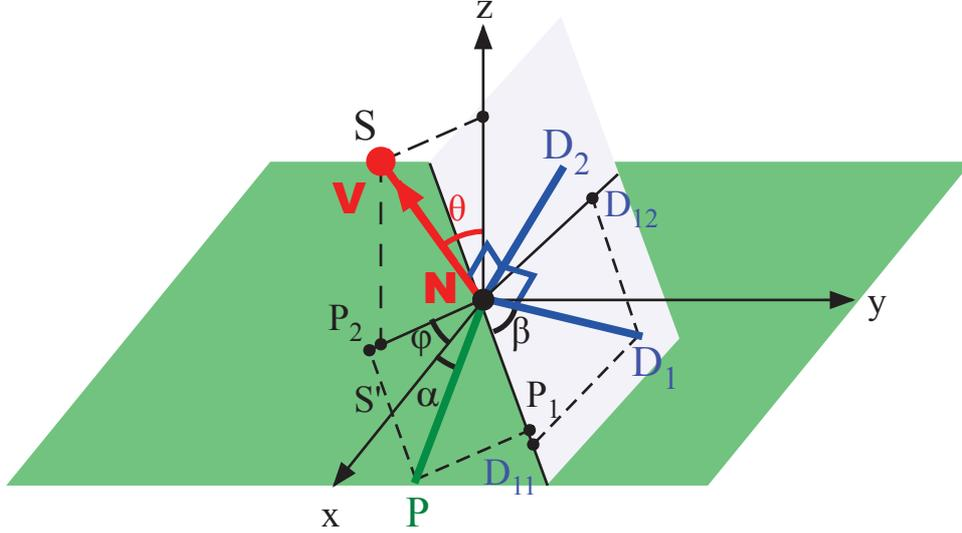
**Figure 8.4:** Modeling of the optical transition dipoles ( $D_1$  and  $D_2$ ) associated to a single NV color center and polarizations.  $D_1$  and  $D_2$  are in the plane perpendicular to NV-axis ( $\mathbf{S}$ ). This plane has a cross-line  $L$  with the  $(x, y)$ -plane (polarization plane).  $P$  represents the polarization of the excitation light and also the polarizer orientation, see 8.1.
