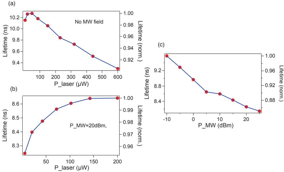
**Figure 6.4:** (a) without applying microwave field, the lifetime of NV color center decreases with excitation laser power. (b) When a ESR resonant microwave field is applied, the lifetime of the NV center increases with the excitation laser power. (c) The lifetime of NV center decreases with microwave power.
