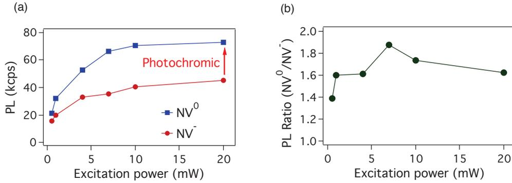
**Figure 2.11:** Figure (a): comparison of emission photon numbers in function of the excitation power, obtained by a single NV color center, in neutral and negative charge states. Figure (b): ratio of emission photons obtained with  $NV^0$  and  $NV^-$  single color centers vs excitation power.
