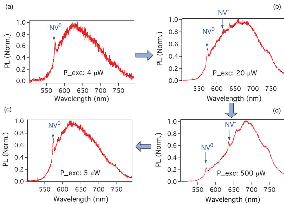
**Figure 2.8:** Reversible photochromic of NV color centers in a CVD bulk diamond as a function of the excitation power.  $P_{exc}$ , the PL spectra red shifts when increase the excitation power, and recovers as soon as the excitation power decreases. The sample contains multiple NV color centers and it is excited by a continuous laser at  $\lambda=532$  nm.
