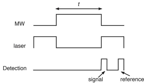
**Figure 6.7:** Pulse sequences for Rabi oscillation. The NV spin is first optically pumped into the  $m_s = 0$  sublevel. Then pulsed microwave radiation is used to coherently manipulate the spin in the dark. Finally, readout is performed by measuring the photoluminescence rate.
