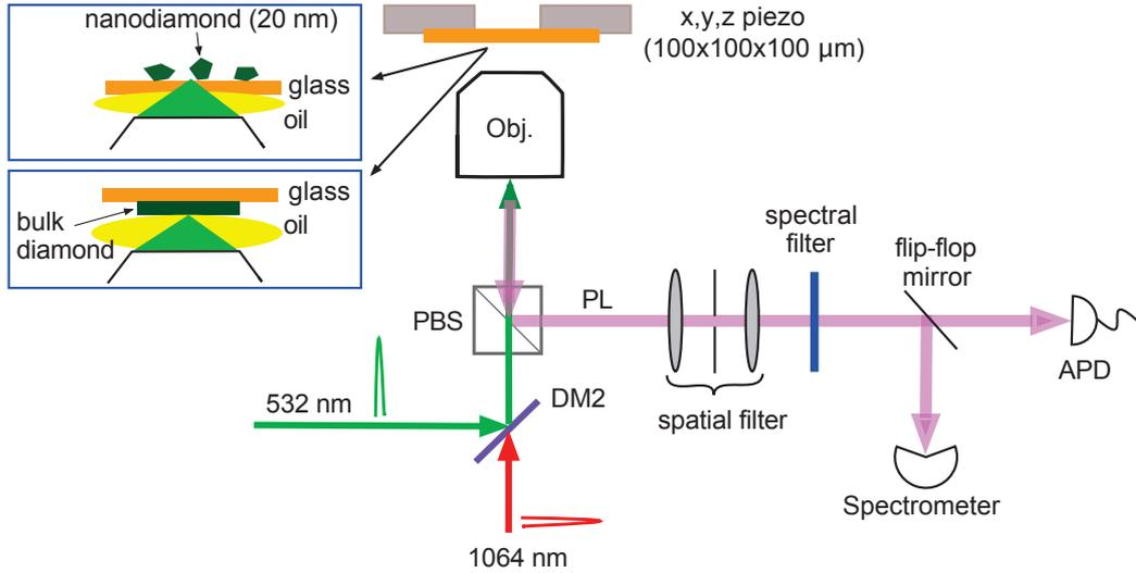
**Figure 3.2:** Experimental setup used to study the effect of IR excitation on the photoluminescence of NV color centers in diamond crystals. The NV color centers are excited, via an oil immersion microscope objective (Obj.), by a pulsed green laser and its photoluminescences are quenched by a pulsed IR excitation. The photoluminescence is collected by the same Obj. and spatially and spectrally filtered before being detected by an avalanche photodiode (APD) or by a spectrometer.
