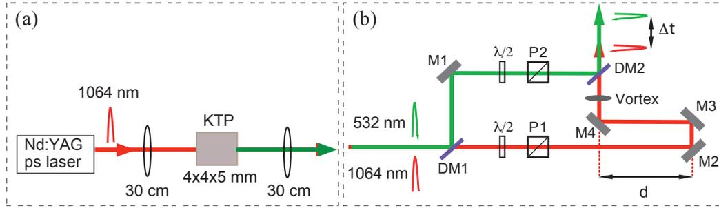
**Figure 3.1:** (a) Pulsed laser source used to excite the NV color centers in diamond. The original mode-locked Nd:VO<sub>4</sub> laser is frequency-doubled providing a synchronized and coherent two-wavelength excitation light source. (b) Experimental setup used to independently control the power and the phase of each laser beam and to vary the time delay between 532 nm and 1064 nm excitation pulses.
