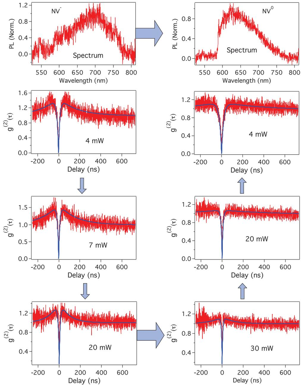
**Figure 2.10:** Photochromic effect of single NV color center in FND, A single  $NV^-$  color center is transformed to a neutral  $NV^0$  charge state after irradiated with 10mW 532nm laser, The irradiation time is more than 5 minutes.
