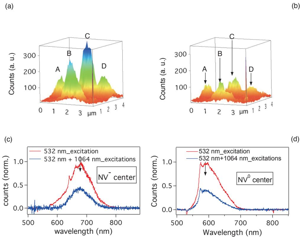
**Figure 3.3:** Effect of pulsed infrared (1064 nm) excitation on the photoluminescence property of NV color centers in diamond nanocrystals. (a) Photoluminescence image obtained with only a 532 nm excitation. (b) Photoluminescence image obtained by simultaneous pulsed excitations at 532 nm and at 1064 nm. (c) and (d) Luminescence spectra obtained without and with infrared excitation for both charge states of NV centers.
