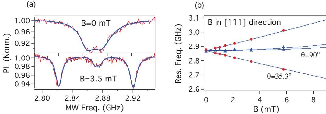
**Figure 7.2:** ESR measurement by increase the  $\mathbf{B}$ -magnitude. (a) When  $\mathbf{B} = 0$ , the ESR resonant frequency is about 2.87 GHz. By increasing  $\mathbf{B}$ -magnitude, the ESR resonant frequency splits due to Zeeman effect, each spin group has special resonance frequency. (b) When the magnetic field is along the [110] orientation, group 1 and 2 are equivalent, meanwhile group 3 and 4 are equivalent.
