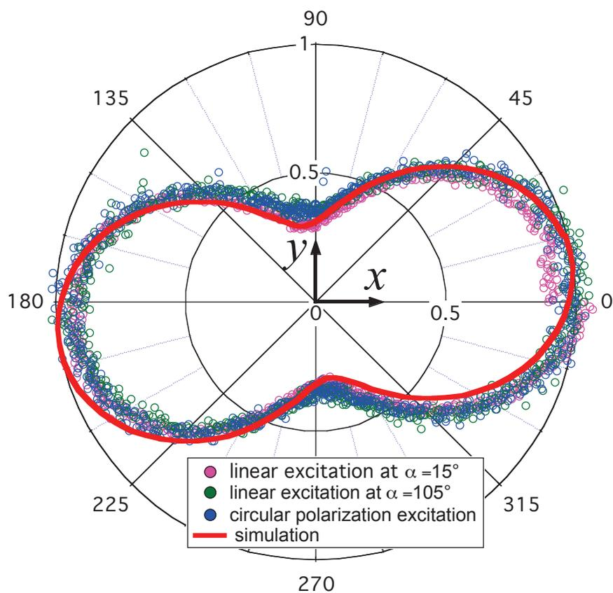
**Figure 8.5:** Normalized NV color center photoluminescence as a function of the analyzing polarizer orientation for three different excitation polarization types. The polarizer is placed in front of the avalanche photodiode and its axis direction is controlled by a rotation motor. The laser excitation power is 0.09 mW.
