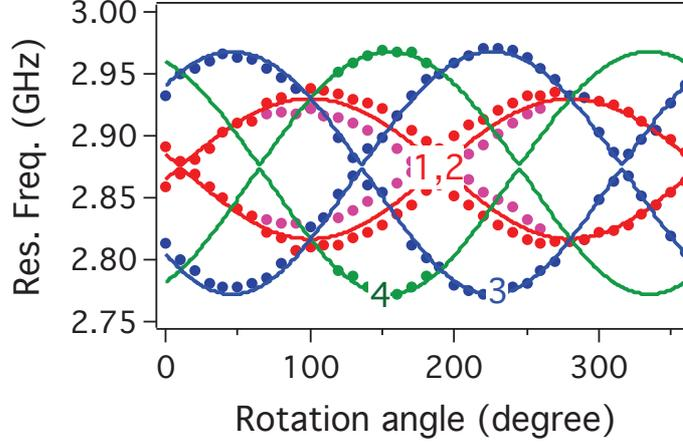
**Figure 7.3:** The ESR spectrum of the ensemble of NV centers in bulk diamond, when the magnetic field is rotate on the [110] surface, group 1 and 2 are equipment, however, group 3 and 4, have  $109^\circ$  phase different, while their amplitude keeps the same.
