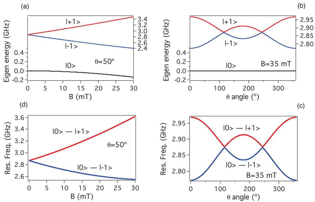
**Figure 5.1:** The calculated energy levels ((a) and (b)) and the resonant frequencies ((c) and (d)) of each states in the presence of a static magnetic field.  $\mathbf{B}$ -magnitude change in (a) and (b),  $\mathbf{B}$  rotates in (b) and (d).
