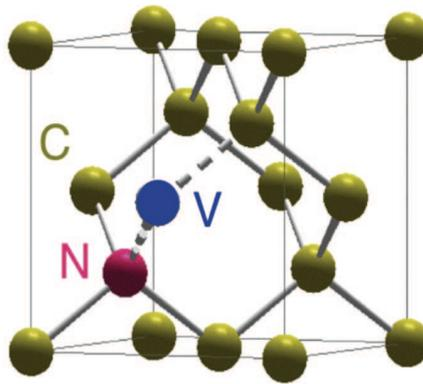
**Figure 2.3:** Schematic representation of the NV center structure.
