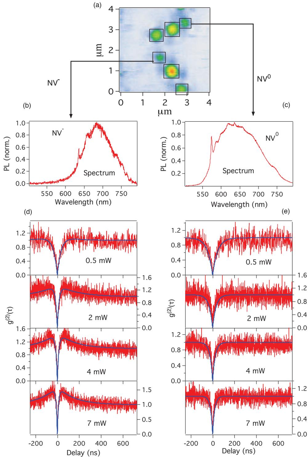
**Figure 2.6:** (a) is the scanning image of diamond nanocrystals containing NV color centers. (b) and (c) are the PL spectrum of a single  $NV^-$  and a single  $NV^0$  color centers, (d) and (e) are the corresponding autocorrelation function measurements. All measurements are realized under the same experimental conditions and at room temperature.
