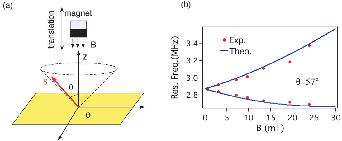
**Figure 8.6:** Determination of the orientation of a single NV spin ( $\mathbf{S}$ ) by ODMR method. First measurement:  $\theta$ -angle is obtained by changing the magnetic field magnitude, which is controlled by translating vertically the magnet along the ( $Oz$ ) axis. ( $x, y$ ) is the sample plane containing also the polarization of the excitation light.
