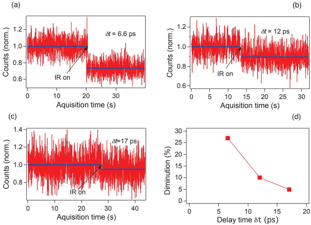
**Figure 3.7:** IR effect on the photoluminescence of NV color center observed when the IR pulses are exposed before VIS pulses. The excitation moment of the IR pulses and the delay time are indicated in each figure. With a delay of 17 ps, no IR effect can be observed. (d) The photoluminescence modulation versus delay time. The solid curves in Figure (a-c) represent the average values which are used to calculate the diminutions.
