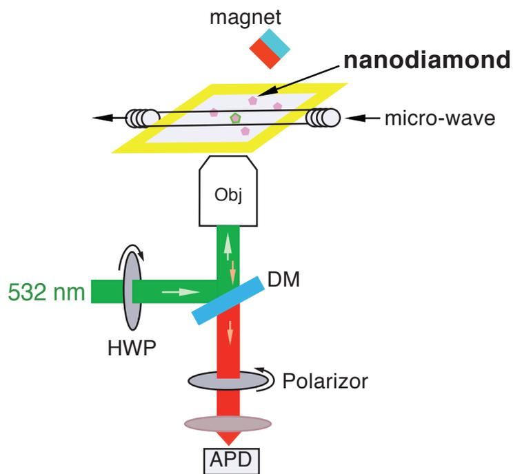
**Figure 8.1:** Experimental setup used to determine the spin orientation and transition dipoles of a single NV color center in diamond nanocrystals. DM: dichroic mirror, high reflection at 532 nm and high transmission in the range 580 – 750 nm. HWP: half-wave plate at 532 nm-wavelength. Obj: microscope objective, numerical aperture  $NA = 0.95$ . The magnet is controlled in orientation and in position by a rotation and a translation systems.
