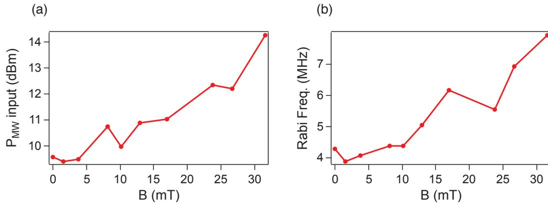
**Figure 6.10:** (a) increasing the magnetic field intensity, in order to have the same output microwave power, the input microwave power is increased. (b) Rabi frequency of NV center as a function of the  $\mathbf{B}$ -magnitude with the input microwave power of Figure (b).
