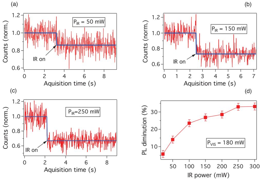
**Figure 3.10:** IR effect on the photoluminescence of NV color centers in bulk diamond. The results are obtained by focusing the IR beam slightly out of the surface of diamond sample. The effect is similar to the one observed with nanodiamonds.
