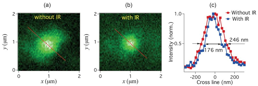
**Figure 4.9:** Optical imaging resolution improvement by IR excitation quenching effect. (a) Scanning image obtained with only a green excitation beam. (b) Scanning image obtained with a combination of a green and an IR doughnut excitation beams. (c) Comparison of the profiles of the photoluminescence spots obtained by two excitation schemes, showing a superresolution of 30 %.
