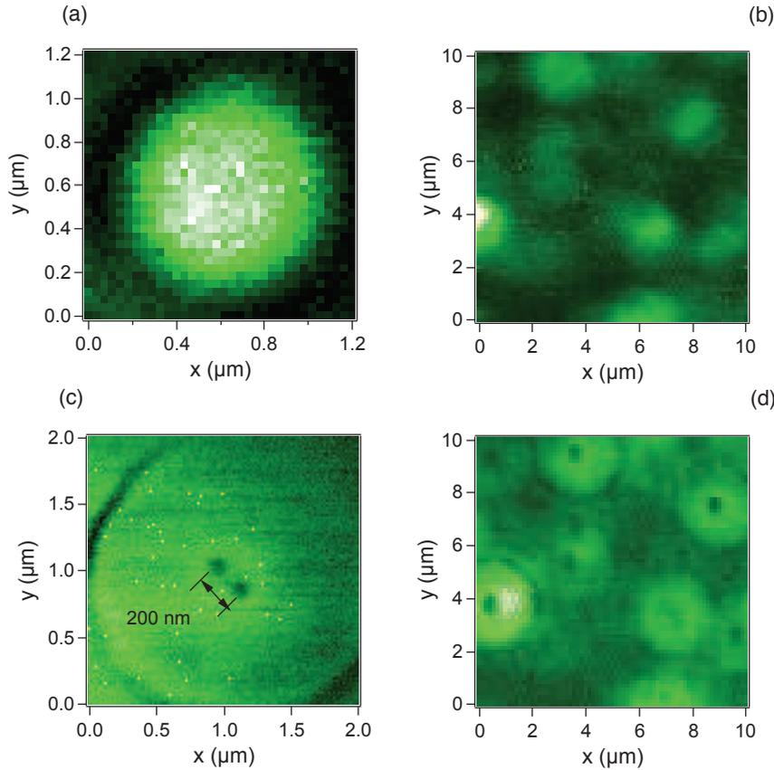
**Figure 4.7:** Super-resolution PL imaging with a doughnut focused spot. (a) and (b) PL images scanned with a gaussian beam. (c) and (d) PL images scanned with a doughnut focused spot. Two NV centers separated by 250 nm which are undistinguished by using a traditional confocal system (a) could be clearly identified (c) by using the douthnut focused spot .
