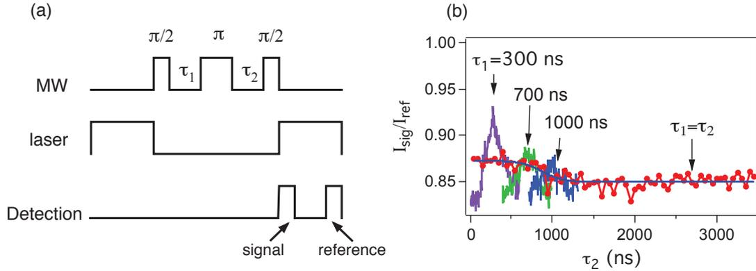
**Figure 6.11:** (a) Pulse sequences for Hahn-echo experiment. (b) Hahn-echo measurement, when fix  $\tau_1$  and change  $\tau_2$  the echo signal is maximum when  $\tau_1 = \tau_2$ . By setting  $\tau_1 = \tau_2 = \tau$  and varying the total free evolution time  $2\tau$ , a decay of the primary echo can be observed.
