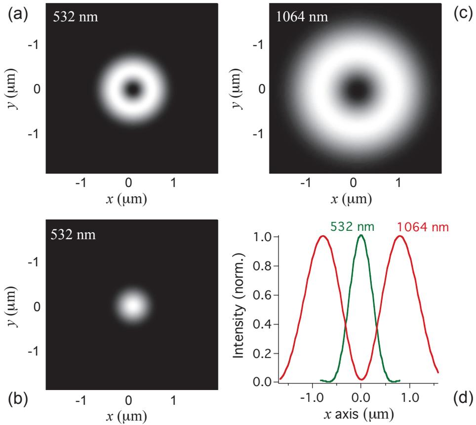
**Figure 4.10:** Theoretical calculation of the Airy and doughnut spots. (a), (b) Doughnut and Airy spots of 532 nm beam, respectively. (c) Doughnut spot of 1064 nm beam. (d) Comparison of the size of the 532 nm Airy spot and 1064 nm doughnut spot. The dark area of the IR doughnut spot is large comparing with the 532 nm Airy spot size. Parameters used for calculations (oil objective microscope): NA (numerical aperture) = 1.4; n (refractive index) = 1.515.
