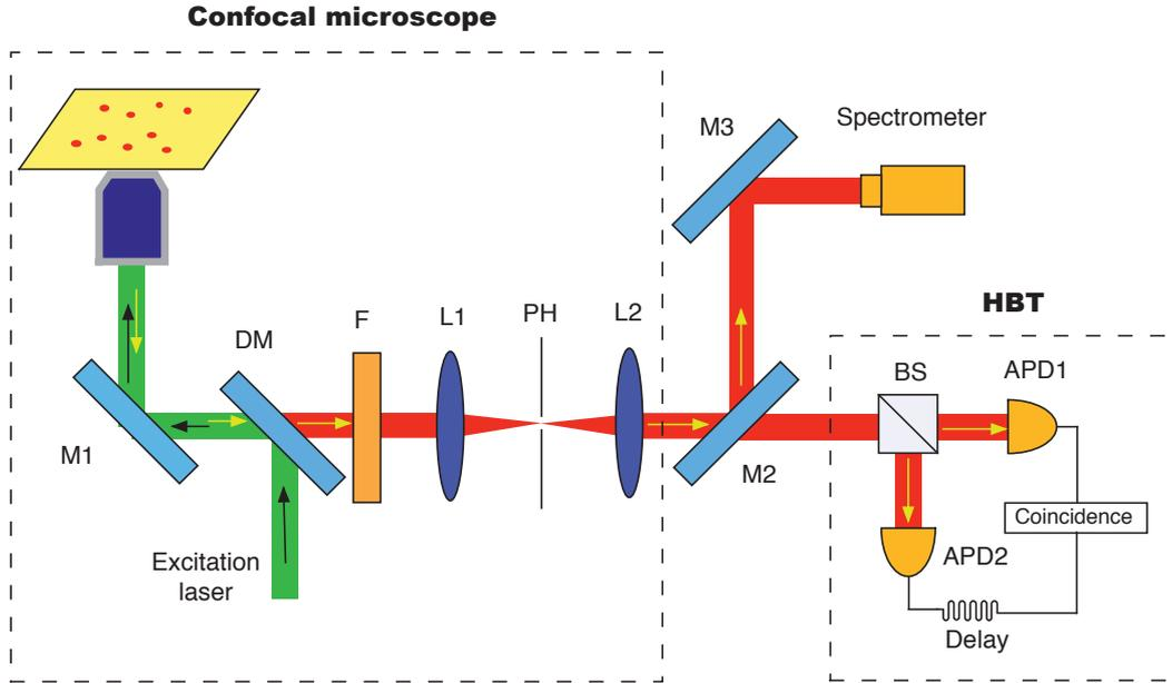
**Figure 2.5:** Optical setup used for detection of PL of NV color center in diamond: M1 is a mirror mounted on a piezoelectric driven tilting system; DM is a dichroic mirror which separates the fluorescence from the excitation light; M2 is a flip-flop mirror for choosing measurement of photon counting (on the avalanche photodiodes APD) or photoluminescence spectrum (using an imaging spectrograph SPC).
