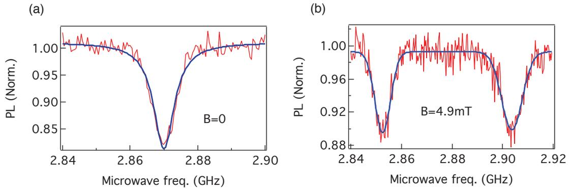
**Figure 5.3:** ESR spectrum of a NV color center, when the microwave frequency (Microwave freq.) is resonant with the NV spin transitions  $m_s = 0 \rightarrow m_s = \pm 1$ , the population is redistributed, and the PL decreases. Figure (a) is ESR spectrum without external magnetic field, the  $|+1\rangle$  and  $|-1\rangle$  state are degenerate. The static magnetic field induces the Zeeman effect and splits the resonance dip into two.
