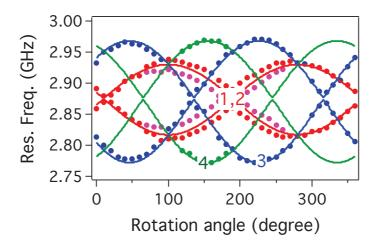
**Figure 7.3:** The ESR spectrum of the ensemble of NV centers in bulk diamond, when the magnetic field is rotate on the [110] surface, group 1 and 2 are equipment, however, group 3 and 4, have 109° phase different, while their amplitude keeps the same.
