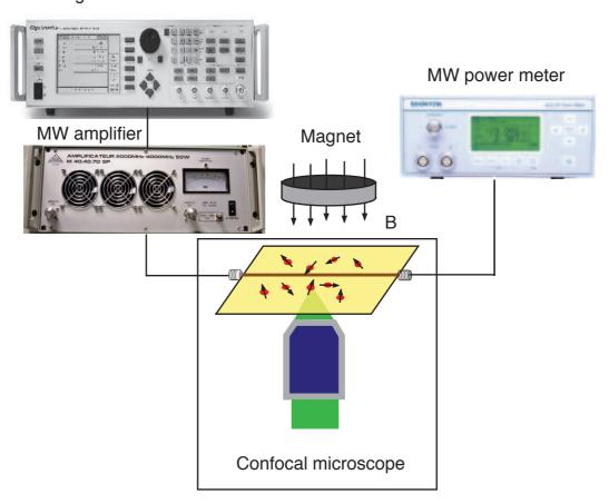
Figure 5.4: The setup for NV spin manipulation, the microwave is sent through a thin copper wire which is close to the sample surface. The magnetic field is applied with a magnet, the magnetic field can be controlled by moving the magnetic in 3D space.
