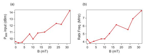
**Figure 6.10:** (a) increasing the magnetic field intensity, in order to have the same output microwave power, the input microwave power is increased. (b) Rabi frequency of NV center as a function of the **B**-magnitude with the input microwave power of Figure (b).
