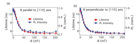
**Figure 7.4:** Measurement of PL intensity and PL lifetime as a function of **B** magnitude. (a) **B** is parallel to the [110] axis. (b) **B** is perpendicular to the [110] axis. The PL intensity changes with a clear correlation with the lifetime modification, both of them decrease obviously with the magnetic field intensity.
