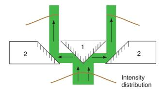
Figure 4.4: A loss free optical system for making an annular beam.
