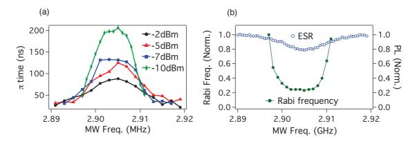
Figure 6.9: (a) Measuring  $\pi$  time of a single NV center when microwave frequency is detuned out of resonance. (b) Rabi frequency of a single NV center when microwave frequency is detuned out of resonance and ESR spectrum.
