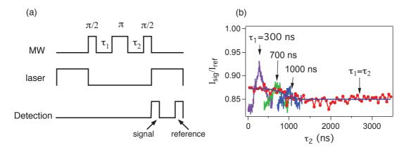
**Figure 6.11:** (a) Pulse sequences for Hahn-echo experiment. (b) Hahn-echo measurement, when fix  $\tau_1$  and change  $\tau_2$  the echo signal is maximum when  $\tau_1 = \tau_2$ . By setting  $\tau_1 = \tau_2 = \tau$  and varying the total free evolution time  $2\tau$ , a decay of the primary echo can be observed.
