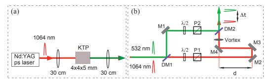
Figure 3.1: (a) Pulsed laser source used to excite the NV color centers in diamond. The original mode-locked  $Nd:VO_4$  laser is frequency-doubled providing a synchronized and coherent two-wavelength excitation light source. (b) Experimental setup used to independently control the power and the phase of each laser beam and to vary the time delay between 532 nm and 1064 nm excitation pulses.
