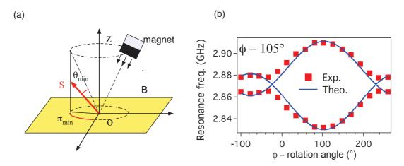
Figure 8.7: Determination of the orientation of a single NV spin (S) by ODMR method. Second measurement: the azimuthal  $\phi$ -angle is obtained by changing the magnetic field (B) orientation. (a) The magnet is rotated horizontally around the Oz-axis while its North-South axis is always pointing towards the NV color center. Doing that, the angle between B and S is changed, and the two resonances frequencies varies as plotted on (b). B-magnitude is kept constant at 3.5 mT.
