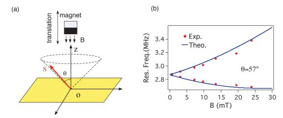
Figure 8.6: Determination of the orientation of a single NV spin (S) by ODMR method. First measurement:  $\theta$ -angle is obtained by changing the magnetic field magnitude, which is controlled by translating vertically the magnet along the (Oz) axis. (x,y) is the sample plane containing also the polarization of the excitation light.
