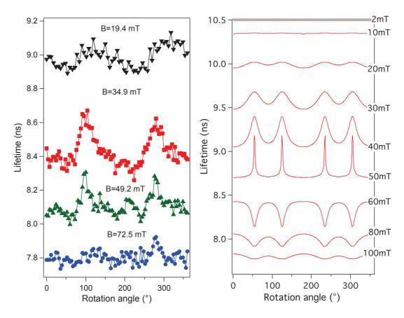
**Figure 7.5:** Lifetime measurement by rotating **B**-orientation on the [110] plane. (a) Experimental result, the measurements of 4 different **B** magnitudes (19.4 mT, 34.9 mT, 49.2mT and 72.5 mT) are made. (b) Calculation result of the ideal case: all the NVs including the density and orientations are uniformly distributed. Lifetime of  $|0\rangle$  and  $|\pm 1\rangle$  states are 10.5 ns and 7 ns respectively.
