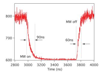
**Figure 5.6:** The instrument response time to the microwave signal. When the microwave signal is switched on the response time is about 90 ns, when the microwave signal is switched on the response time is about 60 ns.
