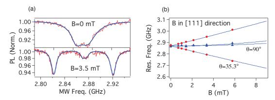
Figure 7.2: ESR measurement by increase the B-magnitude. (a) When  $\mathbf{B}=0$ , the ESR resonant frequency is about 2.87 GHz. By increasing B-magnitude, the ESR resonant frequency splits due to Zeeman effect, each spin group has special resonance frequency. (b) When the magnetic field is along the [110] orientation, group 1 and 2 are equivalent, meanwhile group 3 and 4 are equivalent.
