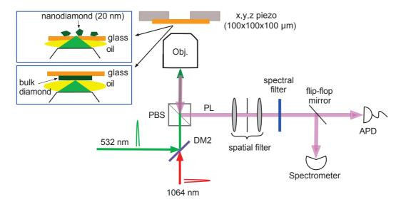
**Figure 3.2:** Experimental setup used to study the effect of IR excitation on the photoluminescence of NV color centers in diamond crystals. The NV color centers are excited, via an oil immersion microscope objective (Obj.), by a pulsed green laser and its photoluminescences are quenched by a pulsed IR excitation. The photoluminescence is collected by the same Obj. and spatially and spectrally filtered before being detected by an avalanche photodiode (APD) or by a spectrometer.
