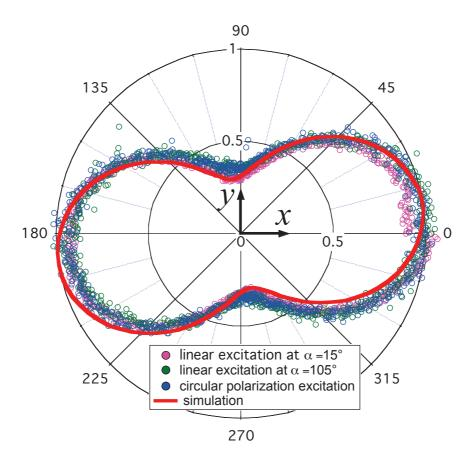
**Figure 8.5:** Normalized NV color center photoluminescence as a function of the analyzing polarizer orientation for three different excitation polarization types. The polarizer is placed in front of the avalanche photodiode and its axis direction is controlled by a rotation motor. The laser excitation power is 0.09 mW.
