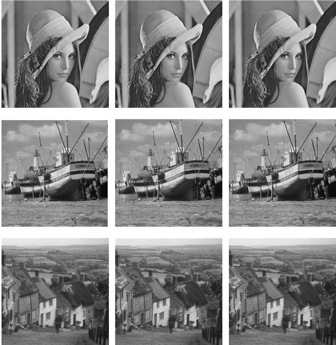
Figure 6.2: From left to right: Original images, halftoned images, reconstructed images. The top image is lena , middle image is boat and bottom image is hill . Even though the halftoned images (center column) perceptually look relatively close to the original images (left column), they are binary. Reconstructed images (right column) are obtained by restoring the halftoned binary images. Best viewed by zooming on a computer screen.
