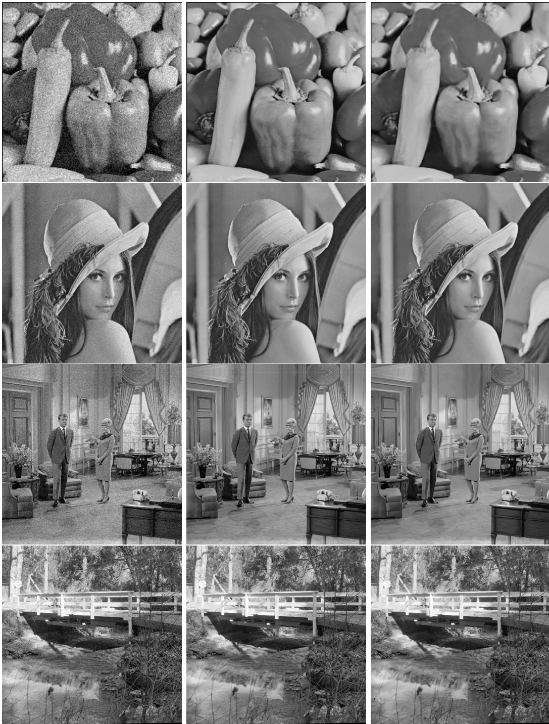
Figure 4.3: Left: noisy images. Middle: Original images. Right: restored images. From top to bottom: peppers image ( \sigma = 20 ), lena image ( \sigma = 10 ), couple image ( \sigma = 15 ), bridge image ( \sigma = 10 ).
