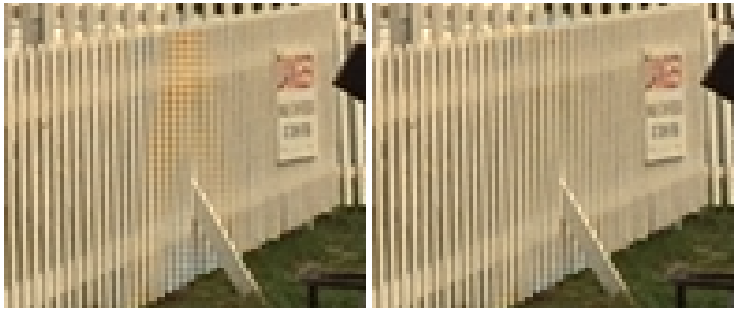
Figure 4.4: Left: Demosaicking with LSC sometimes causes artefacts such as the yellow and blue pixels in the middle of the fence. Right: The reconstruction obtained with the LSSC algorithm does not exhibit such artefacts. (This figure should be viewed in color.)
