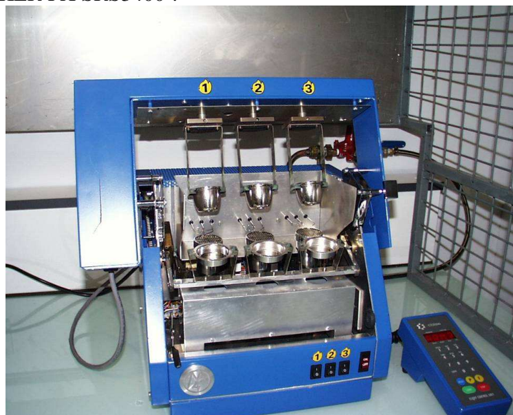
Figure 2A1-1: Equipment of fluxer M4 CLAISSE
