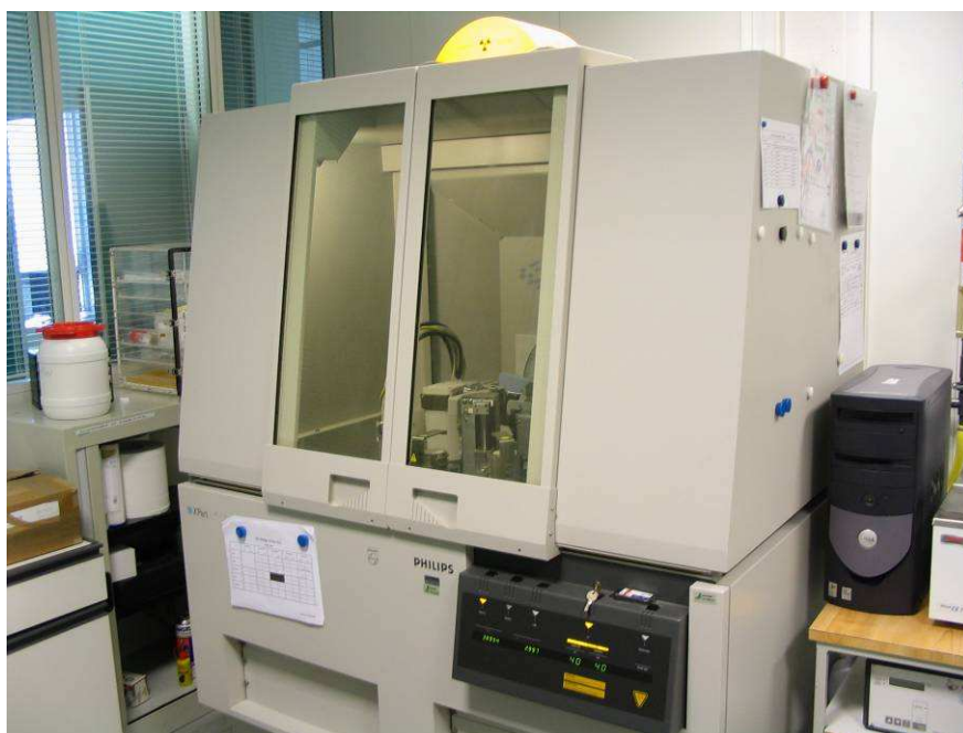
Figure 2A3-2: The equipment of XRD (Philips X'pert)
