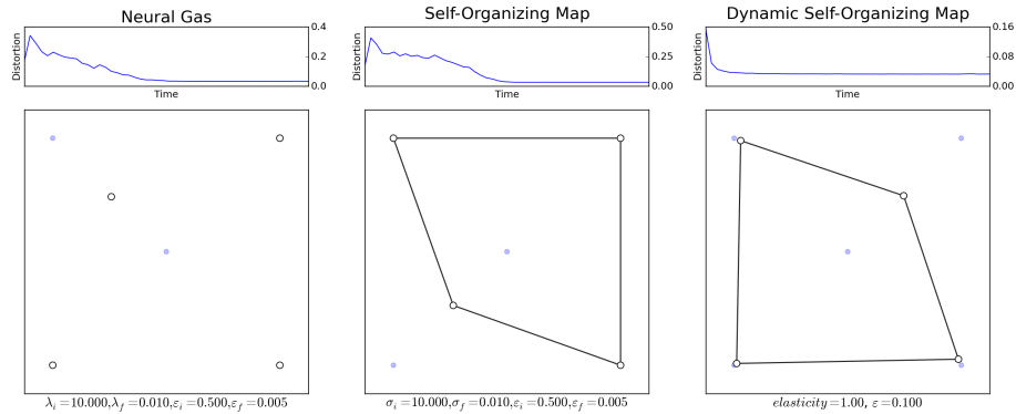
Figure 5: Due to its dynamic nature, the dynamic SOM cannot converge when the number of nodes (4 here) is less than the number of data (5 here). NG and SOM can converge on an approximated solution thanks to both their decaying learning rate and neighborhood and this explains why three nodes are exactly aligned with their corresponding data while the last node found a mid-distance position. In the case of DSOM and because of the constant learning rate, every node is moving at each presented data and thus cannot converge at all.
