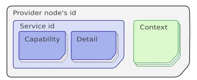
Figure 5.5: Components of a service descriptor message
