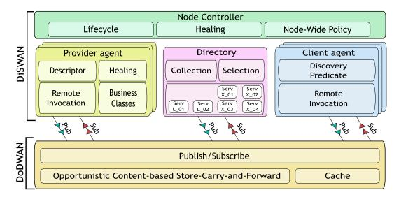
Figure 7.1: Architecture of the service platform
