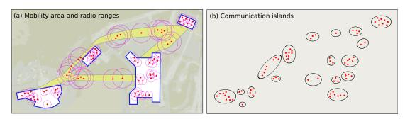
Figure 7.2: Simulation environment of a disconnected MANET. (a) The area represents a university campus where nodes communicate using Wi-Fi in ad hoc mode (radio ranges are illustrated). (b) The network presents disconnected islands of connectivity.
