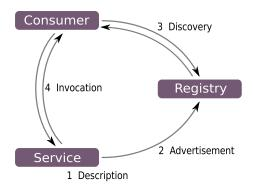
Figure 2.1: Entity interactions in a service oriented architecture
