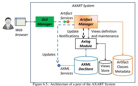
Access control and monitoring queries are handled at the peer level. The architecture of an AXART peer is presented in Figure 6.5.
