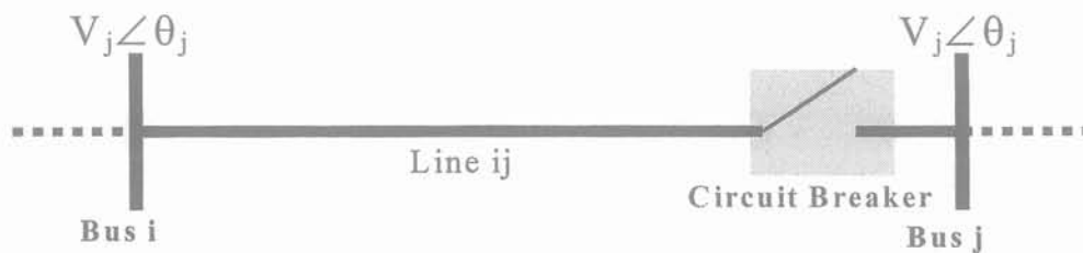
Figure 6.1: SPA difference across the line before closing the circuit breaker ( |\theta_i - \theta_j| )
