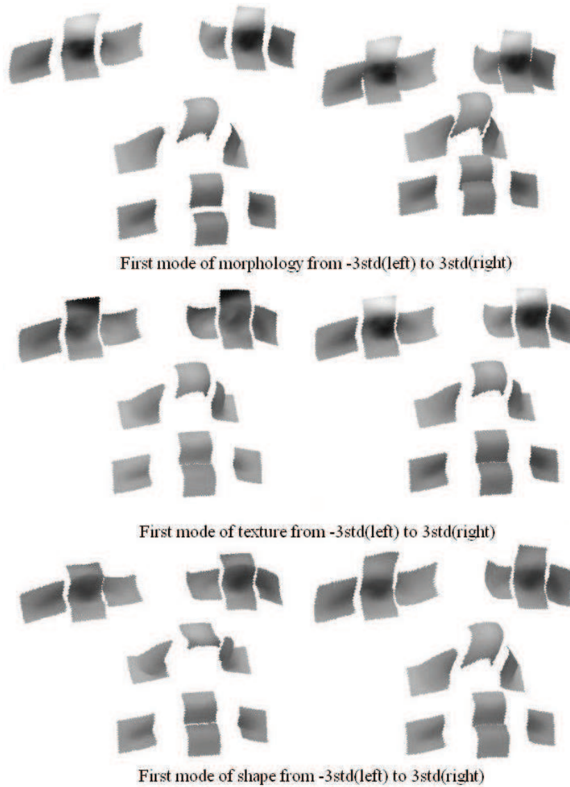
Figure 2.14: SFAM learnt from FRGCv1 dataset: first variation modes on the landmark configuration, local texture and local shape. First mode of morphology explains the landmark configuration variations in terms of face size; first mode of texture explains the intensity variation, especially in the eye region; first mode of shape explains the geometry variation in the upper part of face.
