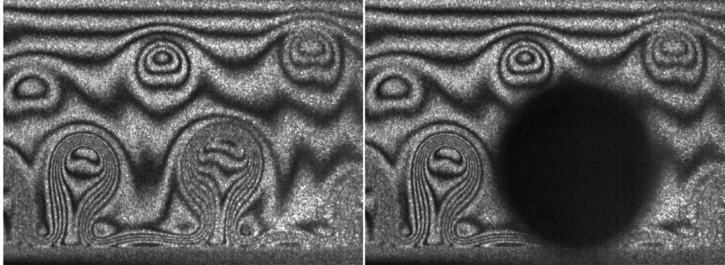
FIGURE 14. Spontaneous bursting at the foot of a flat water film (interferences fringes visualized by a monomode argon laser at 488 nm). Nucleation is seen to occur around a convection cell: the paradigm situation in the bursting of bubbles. Image height is 3 mm and time lapse between both images is 1/3000 s. The film receding velocity is V = 2.8 \text{ m.s}^{-1} corresponding to a thickness h = 20 \mu\text{m} .
