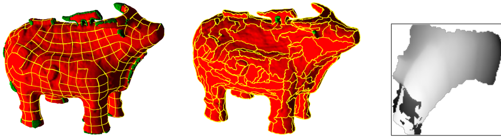
Figure 8.4: Left : Buffle partitioning with PGP, triangles with folding problem have their vertices marked in green. Center : Buffle partitioning with VSA, triangles with folding problem have their vertices marked in green. Right : Example of height map extracted from a chart with a folding problem.
