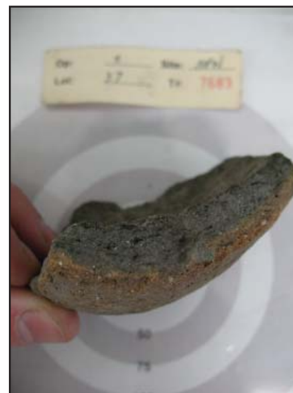
Figure 5.9 - Crucible fragment NPWTC4 cross-section. Image: author.
