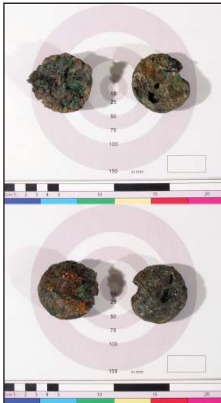
Figure 6.22 - NKHMS19 (top) and inverted (bottom), examples of NKH3/MeP3 ‘slag casts’. Images: author.
