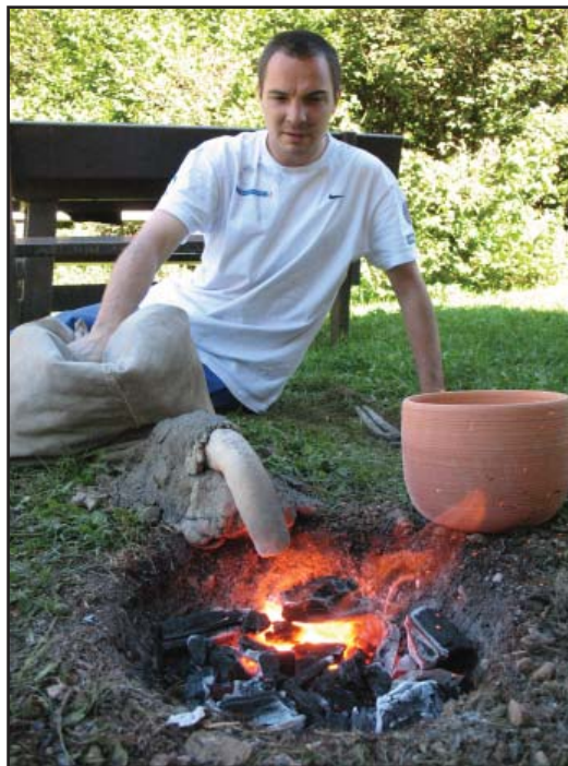
Figure 5.26 - Emilien Burger using forced blast to preheat a charcoal pit prior to a crucible-based copper smelting experiment in Fiaavè, Italy, September 2007. Photo: author.
