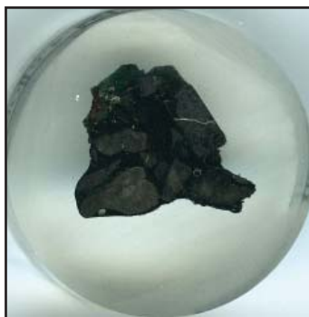
Figure 5.49 - Macroscopically visible residual magnetite in NPWMS6, mounted in 32mm polished block. Image: author.
