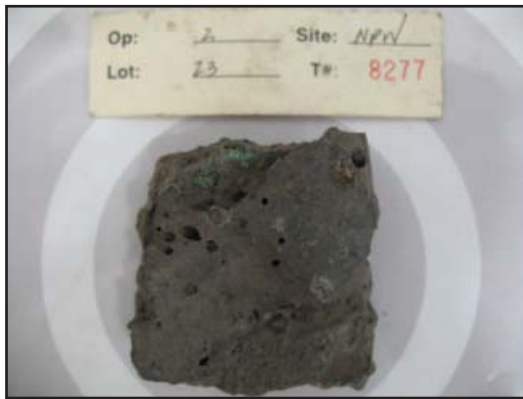
Figure 5.10 - Crucible fragment NPWTC9 slagging. Image: author.
