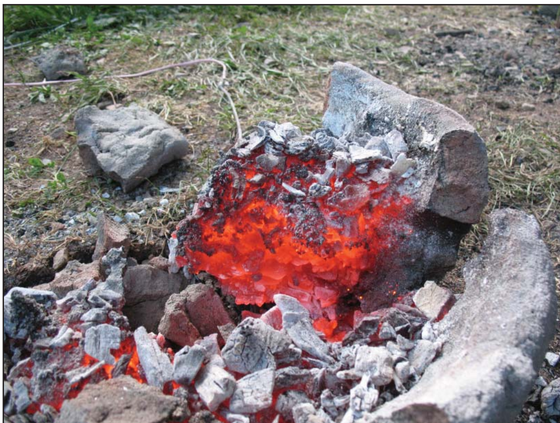
Figure 7.29 - Mass of semi-fused charge attached to the furnace wall during Burn 10. Image: author.
