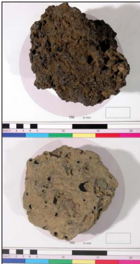
Figure 5.27 - NPWMS6 (top) and NPWMS19 (bottom), examples of NPW3/MeP2 slag cakes. Images: author.
