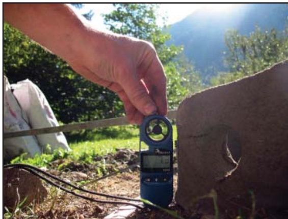
Figure 7.8 - Windspeed at the furnace. Image: author.
