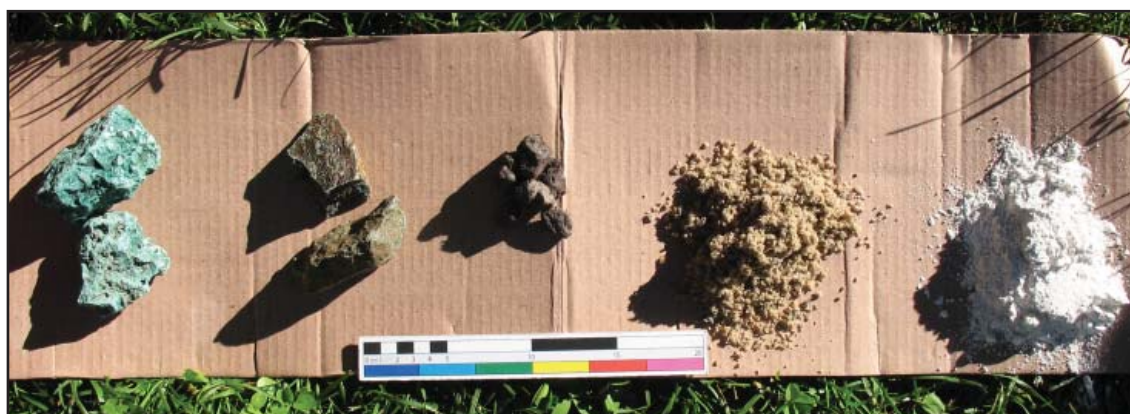
Figure 7.3 - Minerals used in the Fiavè experiments, from left to right: malachite, chalcopyrite, magnetite, quartz, and lime. Image: author.
