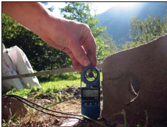
Figure 7.8 - Windspeed at the furnace. Image: author.
