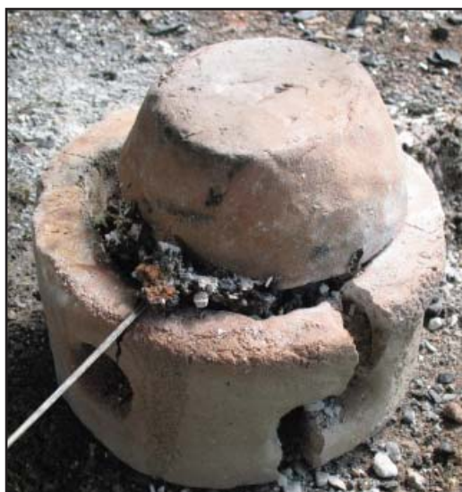
Figure 7.16 - Adhesion of chimney and crucible during Burn 2 - now known to be an archaeologically incorrect association. Image: author.
