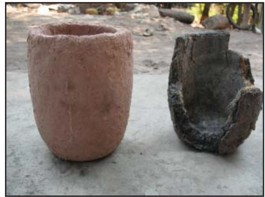
Figure 5.11 - Unused and used brass casting crucibles from Ban Pa Ao. Image: author.
