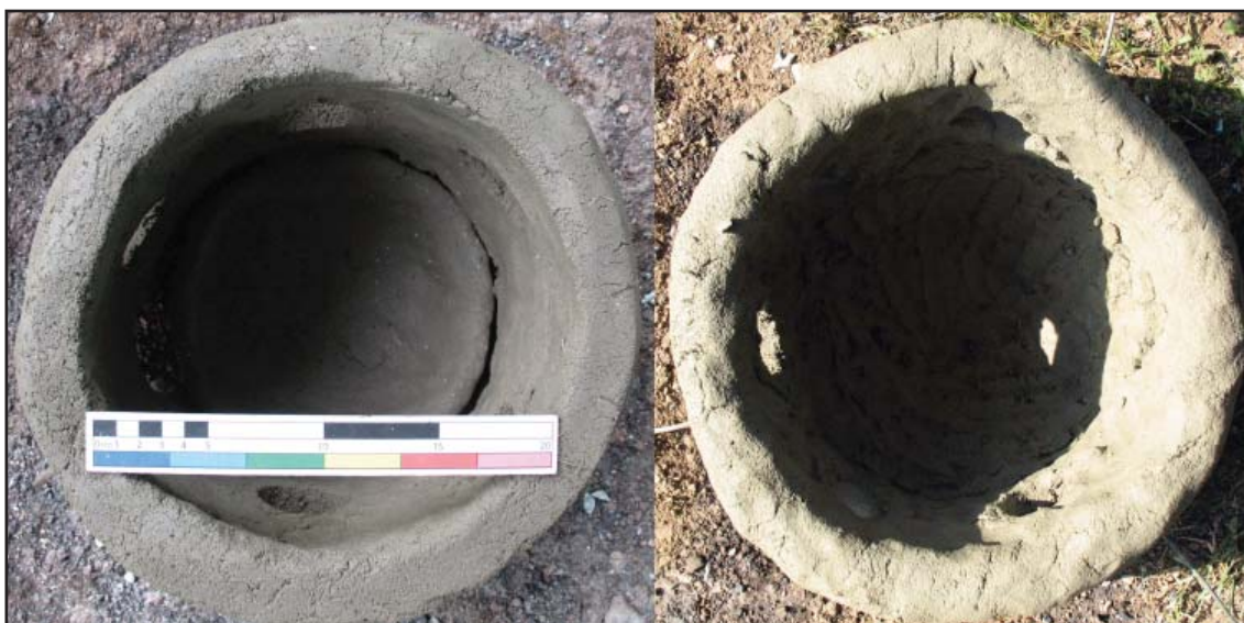
Figure 7.1 - Perforated ceramic cylinder configurations for NPW3/MeP2PR (left) and NKH3/MeP3 (right). Images: author.
