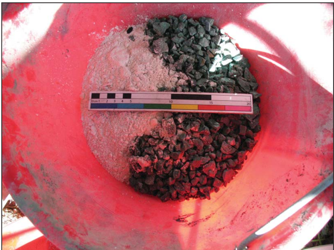
Figure 7.10 - The mineral component of a smelting charge. Image: author.
