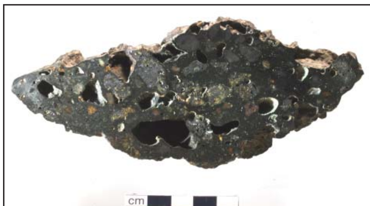
Figure 5.29 - NPWMS7 sectioned and polished to show heterogeneous texture. Image: author.
