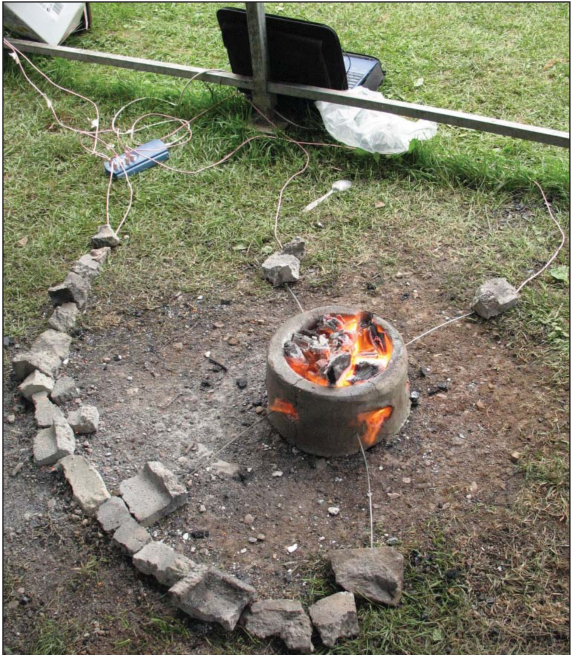
Figure 7.11 - The smelting configuration for ‘Burn 5’. Image: author.
