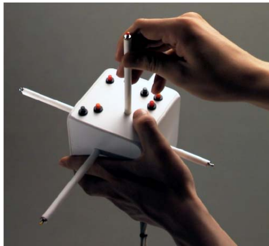
Figure 1.1: The Cubic Mouse Device
