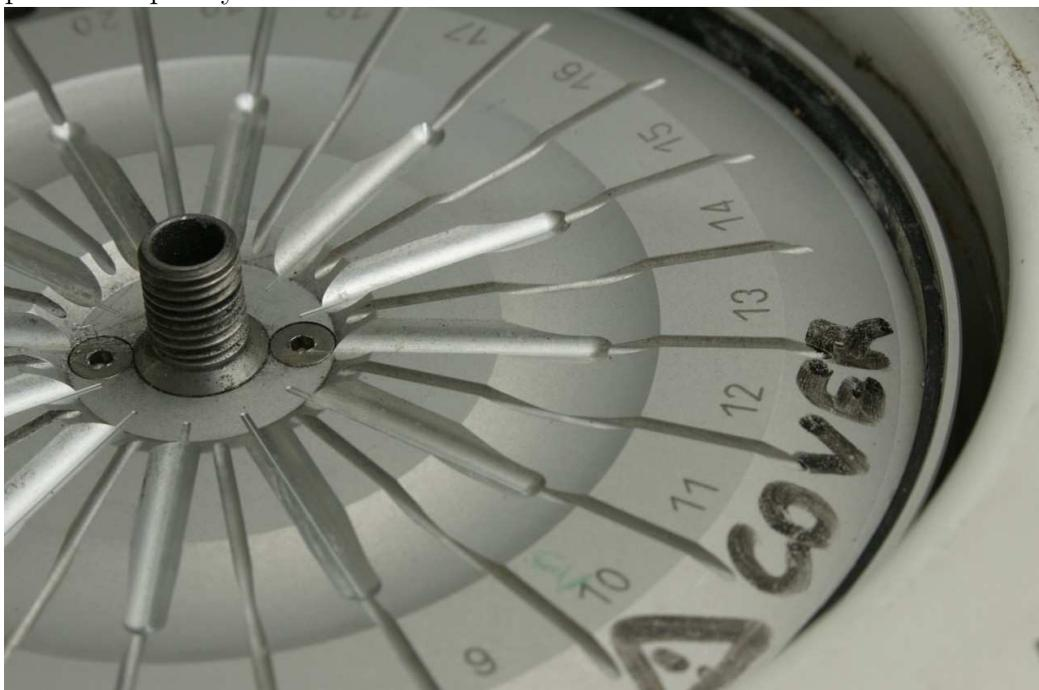
Figure A.5: A capillary centrifuge is used to pack microcrystals to the bottom of the capillary.
