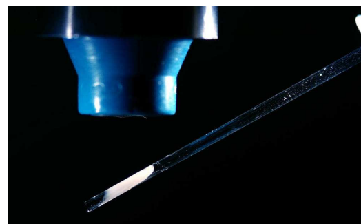
Figure 6.8: Even filled with only 100% glycerol (a classical cryoprotectant), and flash cooled in liquid nitrogen, a white crystalline form of glycerol is formed inside the borosilicate (glass) capillary.
