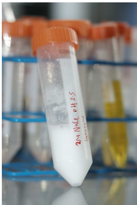
Figure A.2: Though such large volumes are unusual, protein microcrystals can be grown in large quantities by batch crystallisation.
