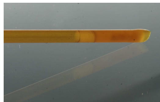
Figure 6.10: While the use of the Sty-cast resin is recommended, it is still possible to use Araldite to seal the capillary. After cycling between cryotemperatures and room temperature, the sample will no longer be sealed. The sample is in white (centre), the araldite is in orange (right side).
