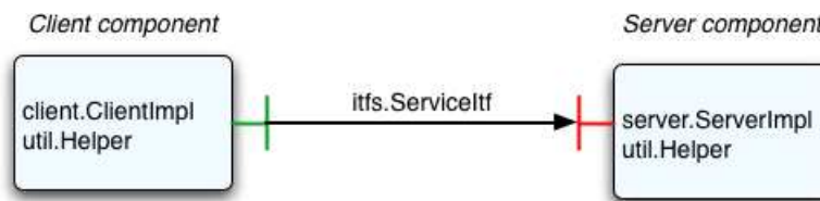
Figure 8.8: A simple client-server component application in Java.
