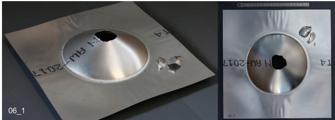
Fig. A2-10. Tested plate 06_1 (0.6 bar)
