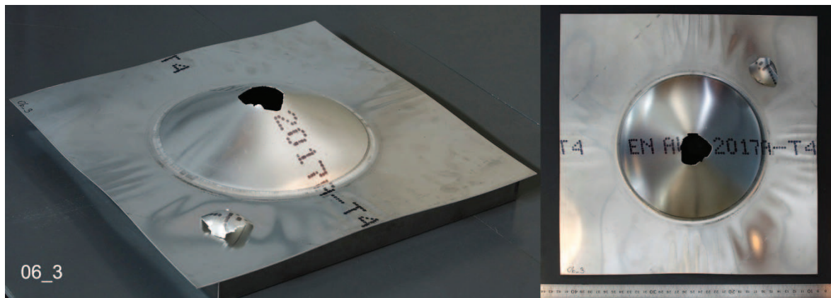
Fig. A2-12. Tested plate 06_3 (0.6 bar)
