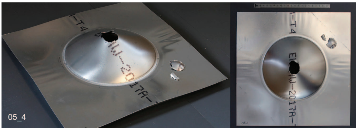
Fig. A2-8. Tested plate 05_4 (0.5 bar)
