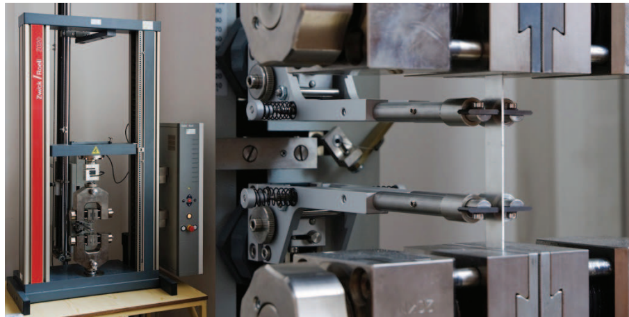
Fig. 4-21. Test machine with the extensometer
