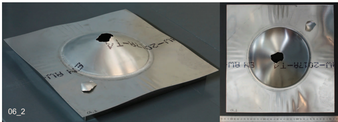
Fig. A2-11. Tested plate 06_2 (0.6 bar)
