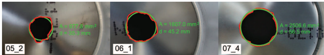
Fig. 4-17. Equivalent hole diameter measurement
