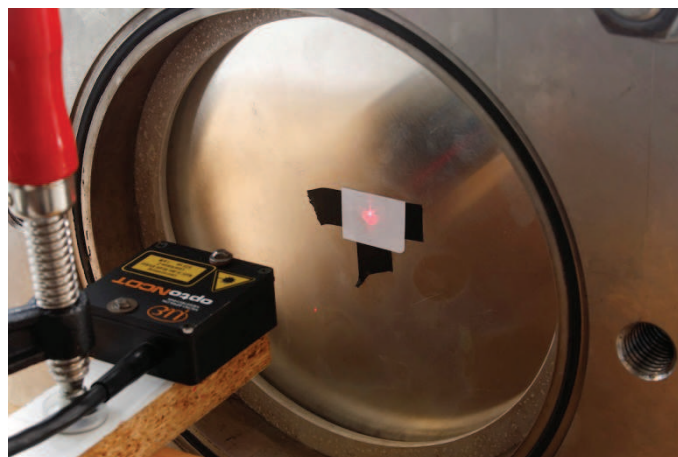
Fig. 4-15. Optic sensor measuring deflection of the plate
