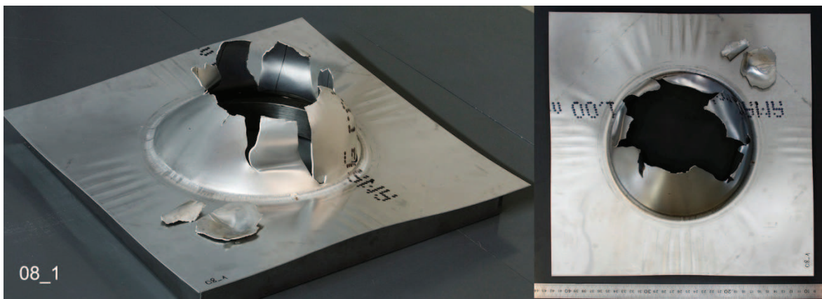
Fig. A2-17. Tested plate 08_1 (0.8 bar)
