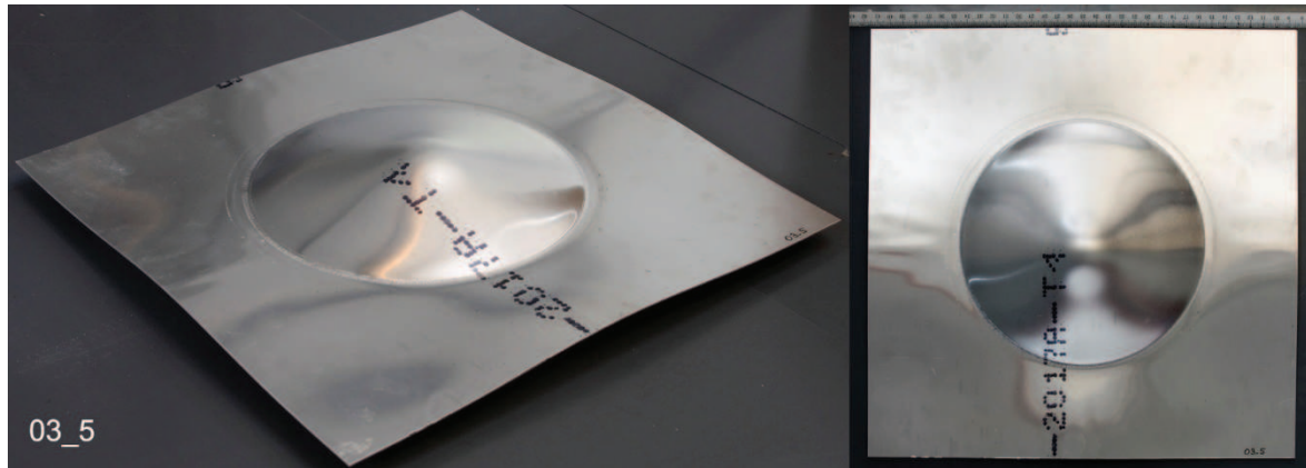
Fig. A2-4. Tested plate 03_5 (0.3 bar)
