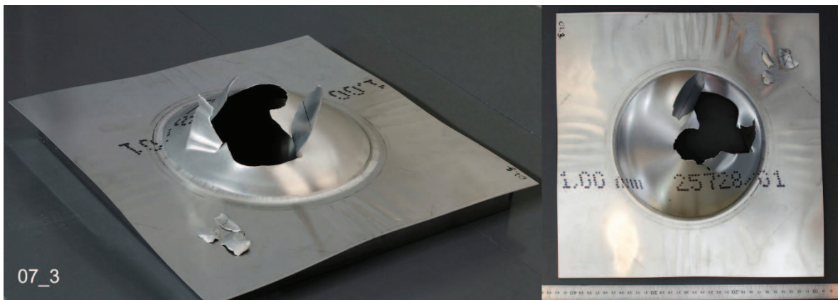
Fig. A2-15. Tested plate 07_3 (0.7 bar)
