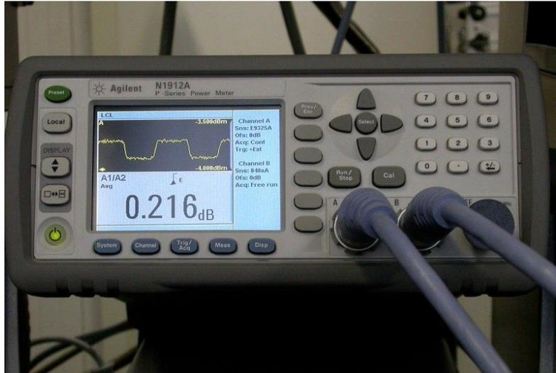
*Figure A.8: The measured Y-factor value displayed with 0.001dB resolution.*
