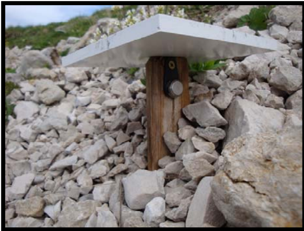
Figure A.3. a) Temperature data logger (the coin is for size comparison); b) the device used to shelter data loggers from direct sunlight.
