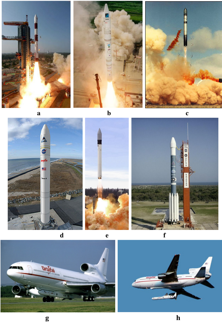
Figure 2.3 – Examples of small satellite launchers: a – first commercial flight of PSLV (credit: ISRO); b – Athena 2 (credit: Lockheed Martin); c – DNEPR; d – Taurus I (credit: Orbital); e – Rockot; f – Delta II (credit: NASA/MSFC); g – Pegasus launcher carried by Lockheed L-1011 “Stargaze”; h – Pegasus XL launching from Lockheed L-1011
