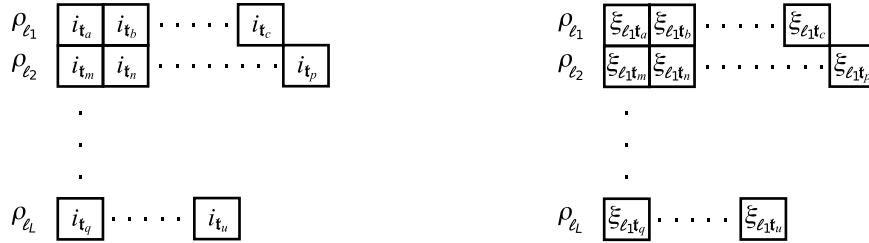
Figure A.3: Indexing of the \xi -coefficients. A list of the transition indices i_{t_j} is constructed for each lower-level multipole \rho_{l_k} . Only exciting transitions from the manifold containing \rho_{l_k} are taken into account for each multipole. At first, the list of the relevant transition indices is constructed (left). Then the coefficients \xi_{t_j} are calculated by the summation over the quantum numbers as described in Subsection 3.3.3 (right).
