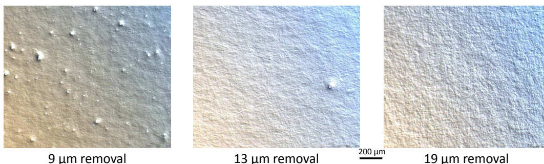
Figure 5.1: Optical microscopy of silicon crystals after different polishing times and consequently different thicknesses removed, measured using an infrared interferometer.
