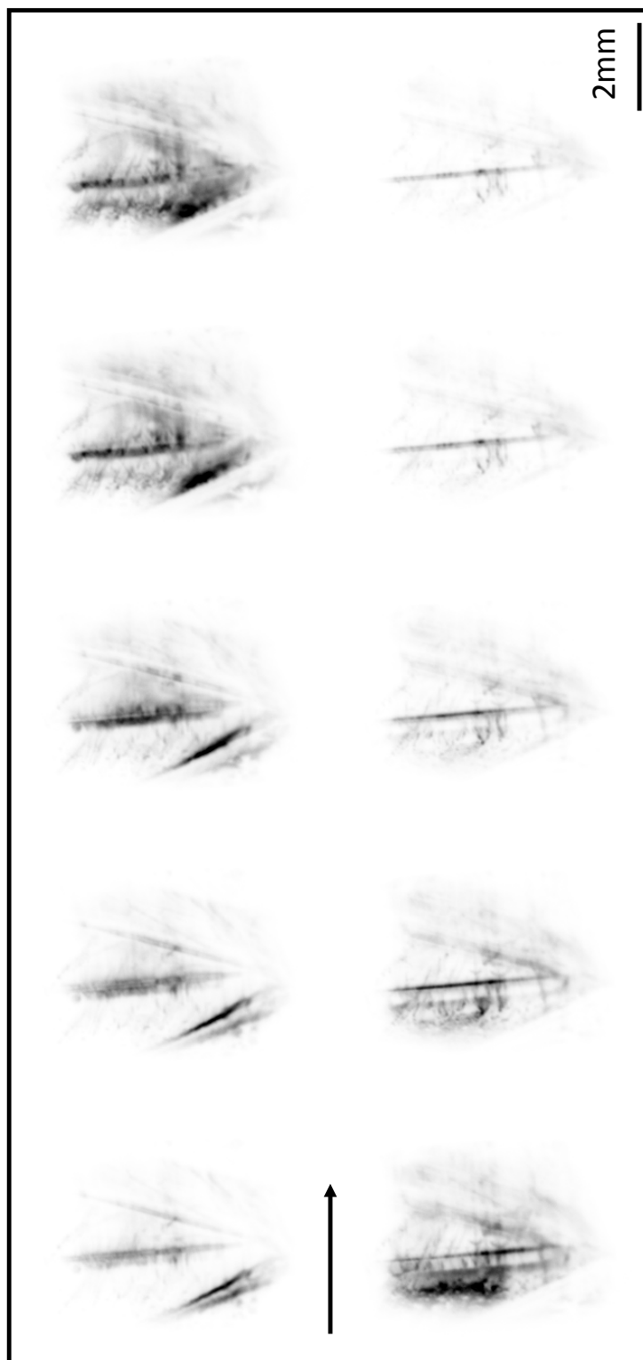
Figure 4.14: Series of topographs in a non-dispersive arrangement taken at ID06 using two diamond crystals, 111 oriented, 333 reflection, monochromatic beam of E=15 keV. The arrow shows the projection of the incident and diffracted wavevectors.
