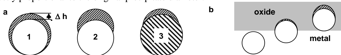
Figure 99: (a) The three sketches show the crack scenarios for different matrix expansion behaviours during oxidation. (1) uniform matrix expansion during oxidation (definition of crack height shown), (2) uniform unidirectional matrix expansion during oxidation and (3) uniform unidirectional matrix expansion during oxidation with isotropic precipitate expansion. (b) The crack height evolution upon incorporation of the precipitate in the oxide is presented. Changes due to different thermal expansion coefficients are not considered.
