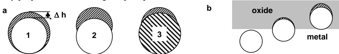
Figure 99: (a) The three sketches show the crack scenarios for different matrix expansion behaviours during oxidation. (1) uniform matrix expansion during oxidation (definition of crack height shown), (2) uniform unidirectional matrix expansion during oxidation and (3) uniform unidirectional matrix expansion during oxidation with isotropic precipitate expansion. (b) The crack height evolution upon incorporation of the precipitate in the oxide is presented. Changes due to different thermal expansion coefficients are not considered.
