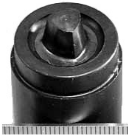
Figure 1.5 – Outil Trivex TM (Copyright ©2001, TWI Ltd) (TNS)
