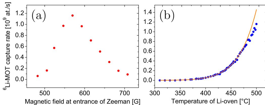
Figure 3.2:  ${}^6\text{Li}$ -MOT capture rate as a function of (a) the axial magnetic field of the Zeeman slower and (b) the temperature of the Li-oven. Circles represent the experimental data and the solid curve the theoretical prediction from Eq. (3.3).
