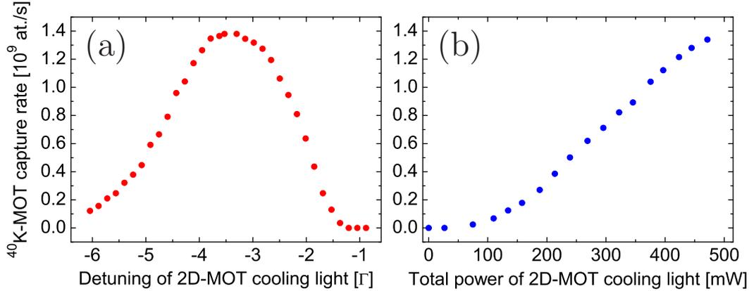
Figure 3.4:  $^{40}\text{K}$ -MOT capture rate as a function of (a) the detuning and (b) the total power of the cooling light used for the 2D-MOT (for a constant intensity ratio between the cooling and repumping light). The total power refers to the sum of the powers in the six 2D-MOT beams, where a power of 470 mW corresponds to a total intensity of  $\sim 47 I_{\text{sat}}$  at the center of the 2D-MOT, with the saturation intensity  $I_{\text{sat}}$  given in Tab. 2.3.
