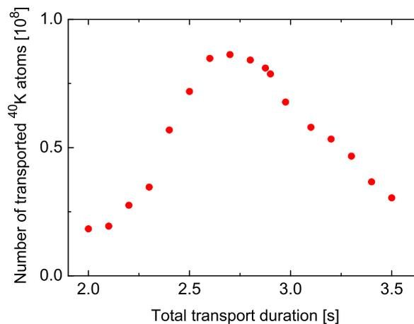
Figure 3.16: Number of magnetically transported atoms as a function of the total transport duration. The initial atom number in the magnetic trap before the transport was  $\sim 5 \times 10^8$  at the day when the graph was recorded.
