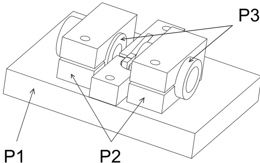
Figure C.8: Schematic of the support for the tapered amplifier chip. The different parts include: a base (P1), collimation tube supports (P2) and the collimation tubes (P3), which are detailed in the subsequent figures. The chosen material for all pieces is duralumin.
