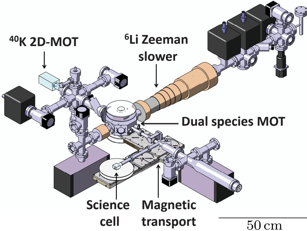
Figure 2.1: Schematics of the vacuum assembly. The dual-species MOT is loaded from a 2D-MOT for  ${}^{40}\text{K}$  and a Zeeman slower for  ${}^6\text{Li}$ . A magnetic transport allows the transfer of the cloud to a UHV science cell with large optical access.
