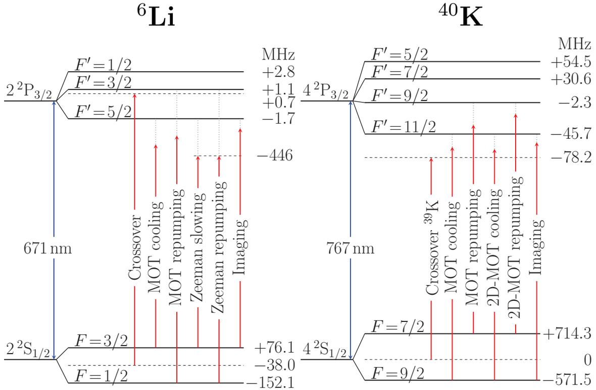
Figure 2.3: Level diagrams for the  ${}^6\text{Li}$  and  ${}^{40}\text{K}$   $D_2$ -lines with their respective hyperfine structures, showing the frequencies required for the dual-species MOT operation. The diode lasers are locked to the indicated saturated absorption crossover signals  $2S_{1/2}(F=1/2, F=3/2) \rightarrow 2P_{3/2}$  of  ${}^6\text{Li}$  and  $4S_{1/2}(F=1, F=2) \rightarrow 4P_{3/2}$  of  ${}^{39}\text{K}$ .
