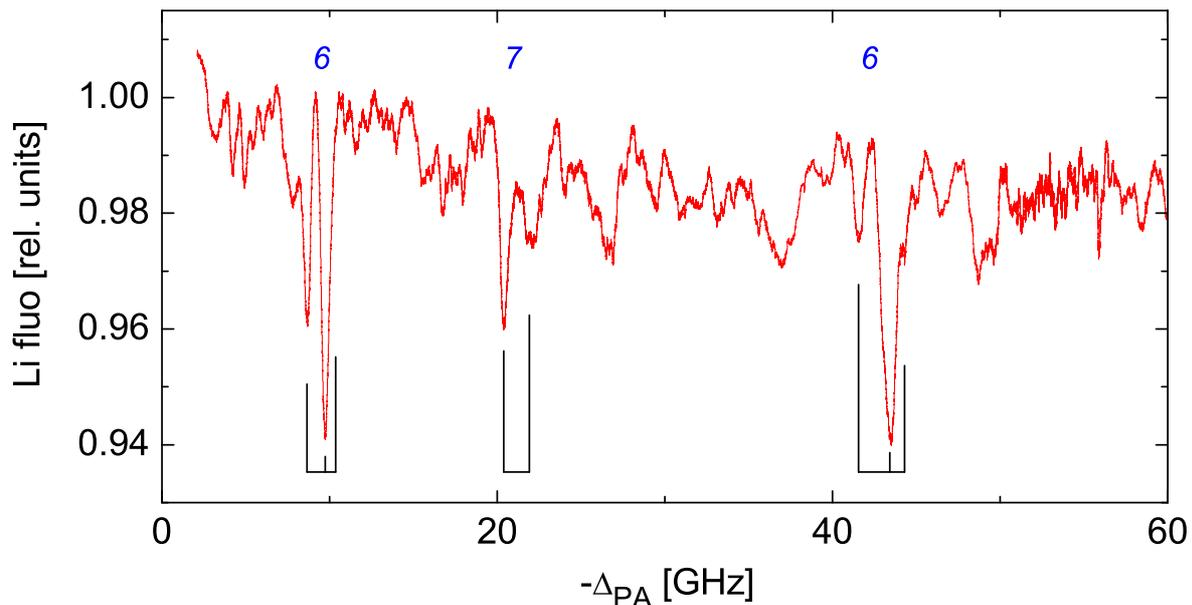
Figure 4.13: Heteronuclear PA trap loss spectrum of  ${}^6\text{Li}{}^{40}\text{K}^*$  below the  $2S_{1/2}+4P_{1/2}$  asymptote. The PA detuning  $\Delta_{\text{PA}}$  is specified relative to the  $4S_{1/2}(F = 9/2) \rightarrow 4P_{1/2}(F' = 9/2)$  transition of  ${}^{40}\text{K}$ . The spectrum contains two vibrational series (labeled  $N = 6, 7$ ) with resolved rotational structure, whose assignment is given in Tab. 4.5.
