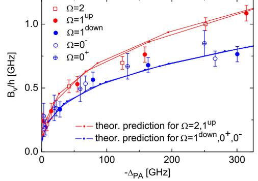
FIG. 4: Measured rotational constants (symbols) for the observed excited molecular states below the  $2S_{1/2}+4P_{3/2}$  asymptote and their theoretical predictions for computed vibrational levels (dots, the lines serve to guide the eye), derived from the potential curves of fig. 1.
