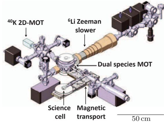
**Fig. 1.** (Color online) Schematics of the vacuum assembly. The dual-species MOT is loaded from a 2D-MOT for  ${}^{40}\text{K}$  and a Zeeman slower for  ${}^6\text{Li}$ . A magnetic transport allows to transfer the cloud to a UHV science cell with large optical access.
