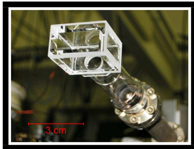
Figure 2.2: Photograph of the ultra-high vacuum science cell in which the ultracold atomic mixture is prepared and investigated. It has to be designed to have a small size in order to provide large mechanical and optical access.
