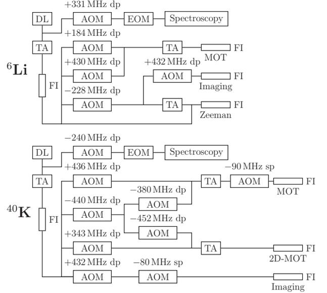
**Fig. 3.** Laser systems for  ${}^6\text{Li}$  and  ${}^{40}\text{K}$ . The frequencies and amplitudes of the various beams are controlled by AOMs in single pass (sp) or double pass (dp) configuration. The EOMs are used to phase modulate a part of the beam for the diode laser's frequency stabilization. Single mode polarization maintaining fibers (FI) are used for beam shaping and spatial filtering. The indicated AOM frequencies allow to generate the required beam frequencies (see Fig. 2).
