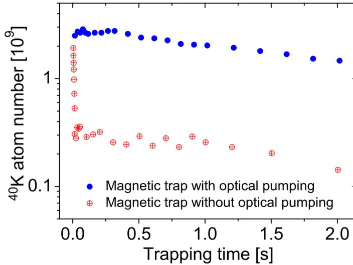
Figure 3.13: Decay curves of the  $^{40}\text{K}$  magnetic trap for the case where optical pumping is applied before the atoms are transferred from the MOT to the magnetic trap and for the case where no optical pumping is applied.
