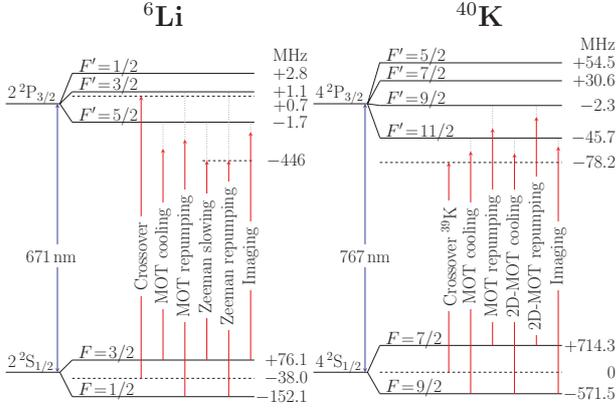
**Fig. 2.** (Color online) Level diagrams for the  ${}^6\text{Li}$  and  ${}^{40}\text{K}$   $D_2$ -lines with their respective hyperfine structures, showing the frequencies required for the dual-species MOT operation. The diode lasers are locked to the indicated saturated absorption crossover signals  $2S_{1/2}(F=1/2, F=3/2) \rightarrow 2P_{3/2}$  of  ${}^6\text{Li}$  and  $4S_{1/2}(F=1, F=2) \rightarrow 4P_{3/2}$  of  ${}^{39}\text{K}$ .
