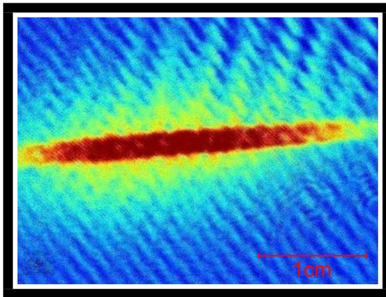
Figure 4.6: Absorption image of the  ${}^{40}\text{K}$ -MOT in presence of the PA beam which is detuned by  $\sim 15$  GHz. The red color represents a spatial region with enhanced density of  ${}^{40}\text{K}$  atoms which results from the attractive optical dipole forces induced by the PA beam. Due to this density enhancement the PA induced heteronuclear losses are expected to be large in this region of PA detunings.
