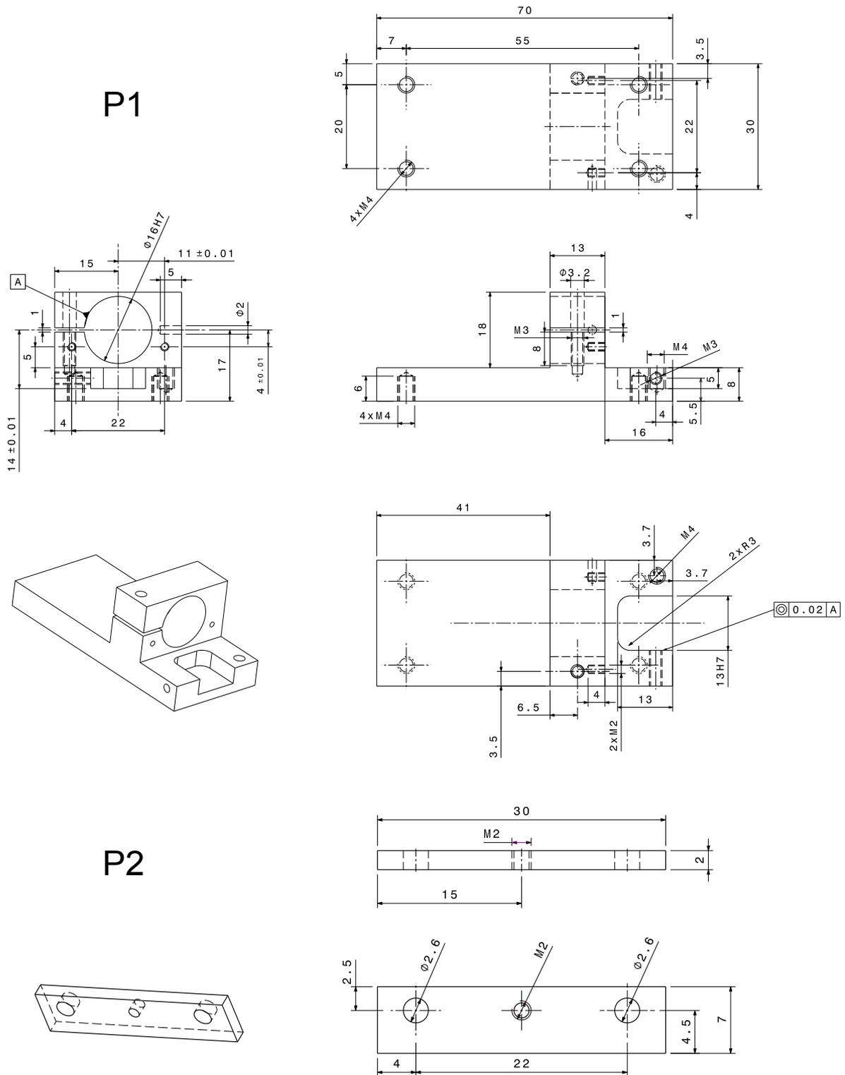
Figure C.4: Engineering drawings of the base (P1) and the laser chip mount (P2). Required precision:  $\pm 0.1$  mm, except as specified otherwise.
