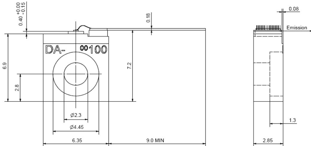
Figure C.2: Engineering drawings of the tapered amplifier chip for potassium (Eagleyard, ref. EYP-RWE-0790-0400-0750-SOT03-0000), to be mounted on the homemade support whose design is detailed in the subsequent figures.
