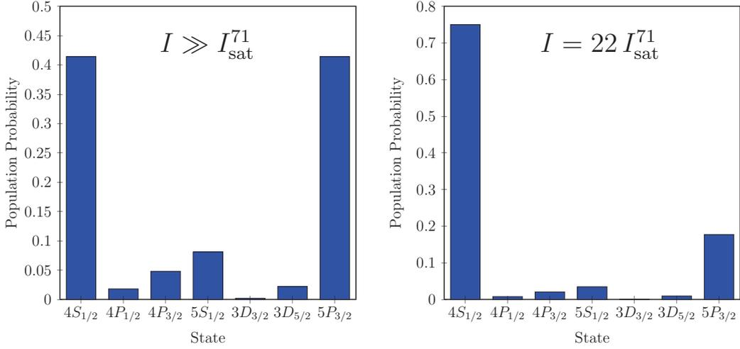
Figure B.4: State population probability for a K-atom that is driven on the violet transition  $4S_{1/2} \rightarrow 5P_{3/2}$  with (left) very large intensity ( $I \gg I_{\text{sat}}^{71}$ ) and (right) the particular intensity  $I = 22 I_{\text{sat}}^{71}$ , for which the atom populates the ground state  $4S_{1/2}$  with a probability of 75%. In a simple two-level atom approximation, this population probability would be expected for  $I = I_{\text{sat}}^{71}$ .
