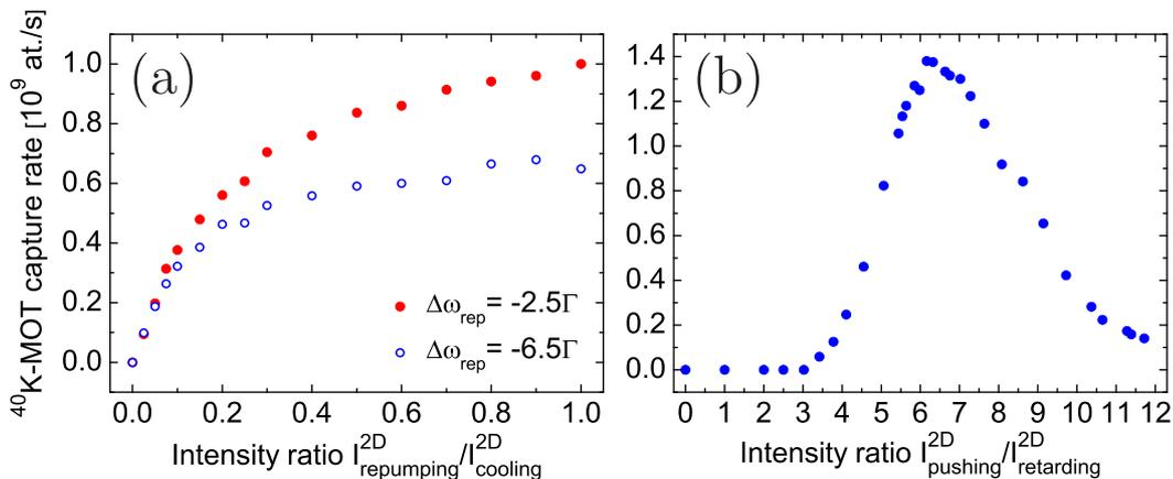
Figure 3.5:  $^{40}\text{K}$ -MOT capture rate as a function of the intensity ratio between (a) repumping and cooling light of the 2D-MOT for two different repumping detunings  $\Delta\omega_{\text{rep}}$  and a constant total cooling light power of 300 mW (which corresponds to a total intensity of  $\sim 30 I_{\text{sat}}$ ) and (b) the pushing and the retarding beams of the 2D-MOT. The intensities of the pushing and retarding beams refer to the intensities along the atomic beam axis.
