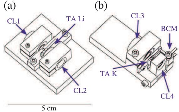
**Fig. 17.** (Color online) Sketch of the tapered amplifier supports for (a) Li and (b) K. In the figure, TA Li and TA K refer to the respective tapered amplifier chips, CL1, CL2, CL3 and CL4 to the (only longitudinally adjustable) collimation lens supports and BCM to the isolated mount for the blade connectors used to power the chip for K. The supports for the output collimation lenses are CL2 and CL4.
