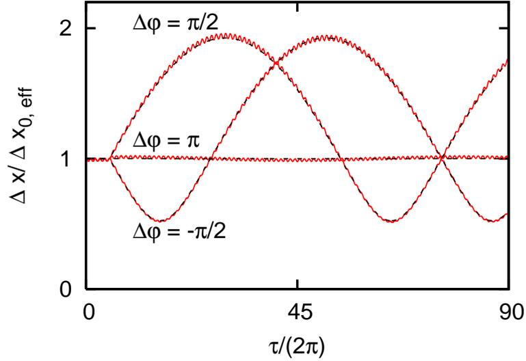
Figure 5.6: Time-evolution of the rms-deviation  $\Delta x$  for a particle in the Paul-trap (5.2) which initially is in the mean-motion ground state, affected by a phase hop of different sizes  $\Delta\varphi$  (normalized to the theoretically predicted initial mean-motion value  $\Delta x_{0,\text{eff}} = \sqrt{\hbar/(2m\Omega)}$ ). Solid (red) curves: results of numerical simulations, dashed (black) curves: theoretical mean-motion prediction. Driving frequency:  $\omega \approx 70\Omega$ .
