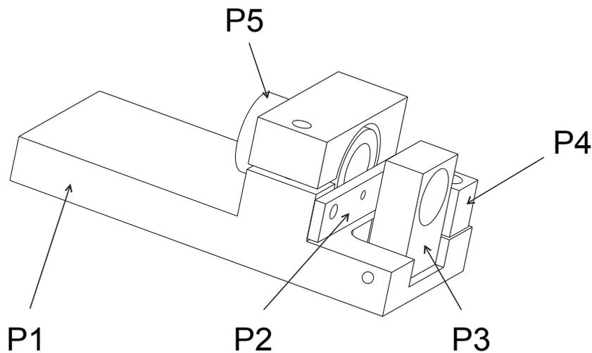
Figure C.3: Schematic of the support for the tapered amplifier chip. The different parts include: a base (P1), a laser chip support (P2) and mounts for the output collimation lens (P3), the isolated blade connectors (P4) and the input collimation lens (P5), which are detailed in the subsequent figures. The chosen materials are: duralumin (P1), copper (P2, P3, P5) and teflon (P4).
