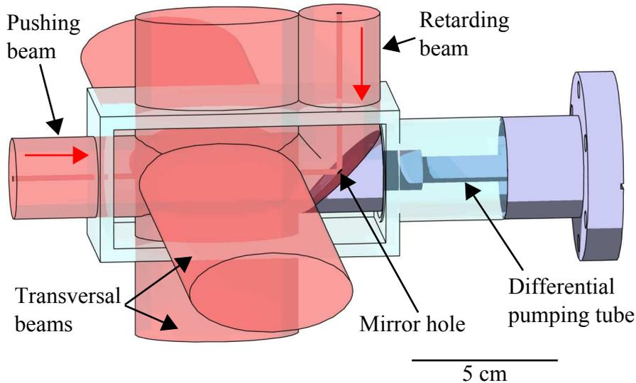
Figure 2.9: Sketch of the parallelepipedal glass cell used for the  $^{40}\text{K}$  2D-MOT. A mirror is placed inside the vacuum chamber to allow an independent control over the longitudinal beam pair. The mirror has a hole in its center and creates a dark cylindrical region in the reflected beams.
