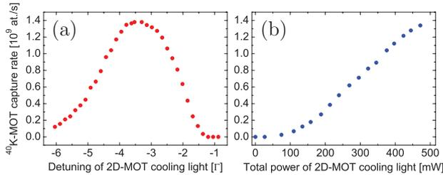
**Fig. 8.** (Color online)  $^{40}\text{K}$ -MOT capture rate as a function of (a) the detuning and (b) the total power of the cooling light used for the 2D-MOT (for a constant intensity ratio between the cooling and repumping light). The total power refers to the sum of the powers in the six 2D-MOT beams, where a power of 470 mW corresponds to a total intensity of  $\sim 47 I_{\text{sat}}$  at the center of the 2D-MOT, with the saturation intensity  $I_{\text{sat}}$  given in Table 3.
