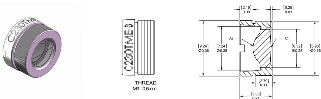
Figure C.6: Engineering drawings of the collimation lens socket (Thorlabs, ref. C230TME-B), to be screwed into the mounts P3 and P5 (entirely).
