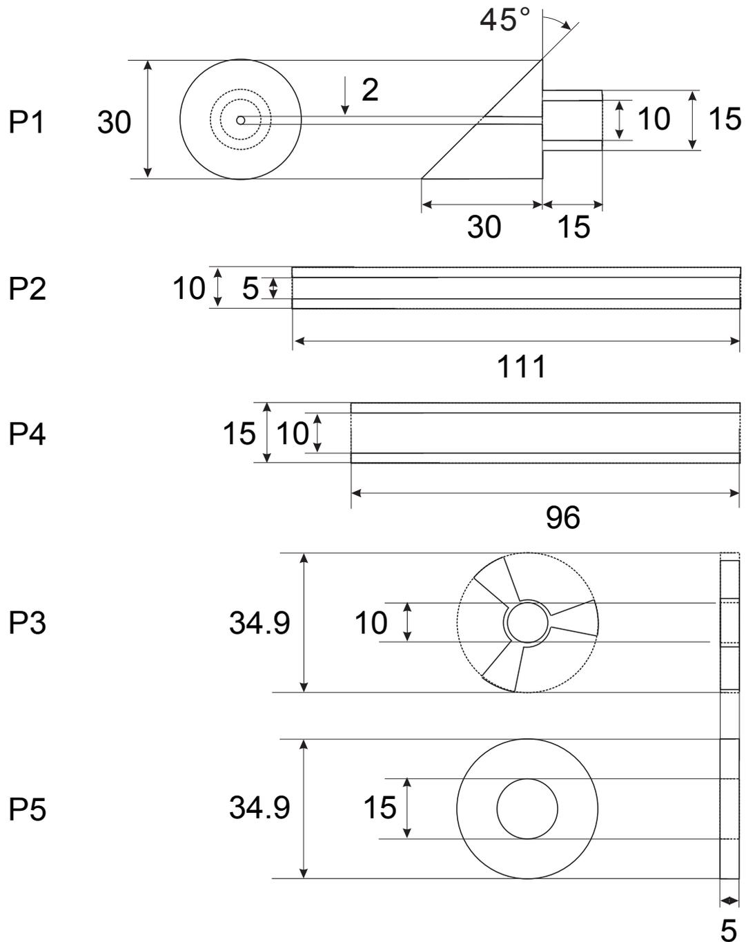
Figure C.11: Engineering drawings of the homemade pieces, *i.e.* the mirror (P1), the first differential pumping tube (P2), the first support ring (P3), the second differential pumping tube (P4) and the second support ring (P5). The material is of type 304.
