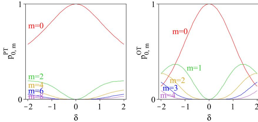
Figure 5.4: The experimentally measurable [233, 234] probabilities for the transitions between the mean-motion ground state  $\phi_0$  and the mean-motion states  $\phi_m$  induced by a phase hop for a particle in the Paul-trap (5.43) (left) and the rapidly scanning optical tweezers (5.45) (right, with  $\omega = \omega_{\text{ref}}$ ) as a function of the parameter  $\delta = \sin(\tau_{\text{ph}} + \Delta\varphi) - \sin(\tau_{\text{ph}})$ .
