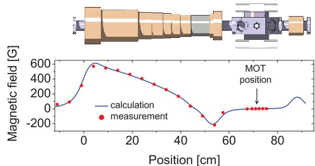
**Fig. 4.** (Color online)  ${}^6\text{Li}$  Zeeman slower coil assembly and generated axial magnetic field profile. The thermal atoms coming from the  ${}^6\text{Li}$ -oven enter the coil assembly at the position 0, and a fraction of them is slowed down and finally captured in the  ${}^6\text{Li}$ -MOT, which is located at 71.4 cm. A compensation coil placed on the opposite side of the MOT (at 84.1 cm) ensures that the magnetic field is zero at the position of the MOT.
