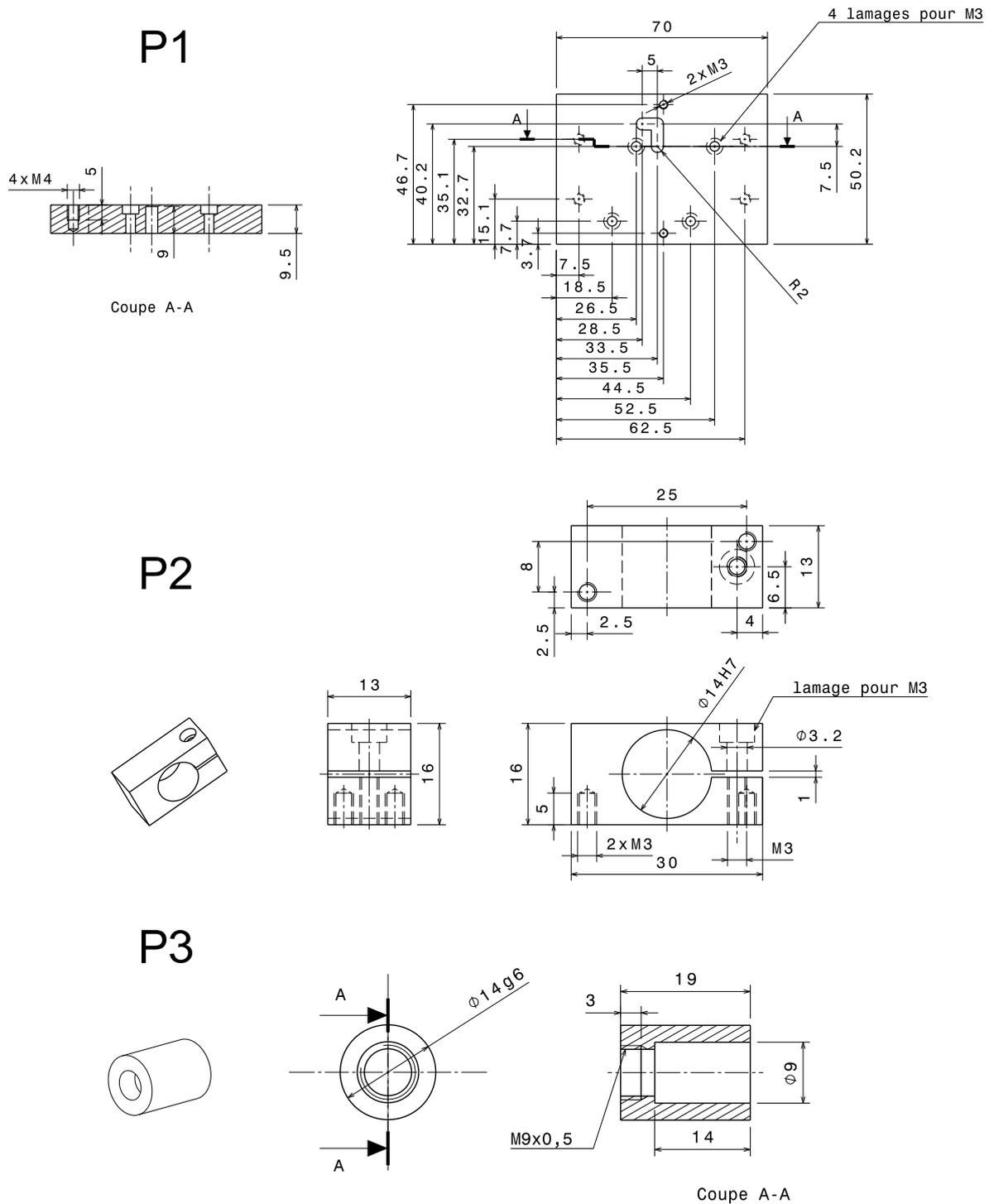
Figure C.9: Engineering drawings of the base (P1), the collimation tube supports (P2) and the collimation tubes (P3). Required precision:  $\pm 0.1$  mm, except specified otherwise. The dimensions of the collimation lenses are given in Fig. C.6.
