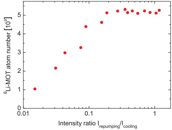
**Fig. 15.** (Color online)  $^6\text{Li}$ -MOT atom number as a function of the intensity ratio between repumping and cooling light for a constant cooling light power of 11 mW per MOT beam (which corresponds to an intensity of  $2 I_{\text{sat}}$ ). In comparison to  $^{40}\text{K}$  (Fig. 13), the optimum atom number requires a larger intensity in the repumping light, which is a consequence of the unresolved excited hyperfine structure of  $^6\text{Li}$ .
