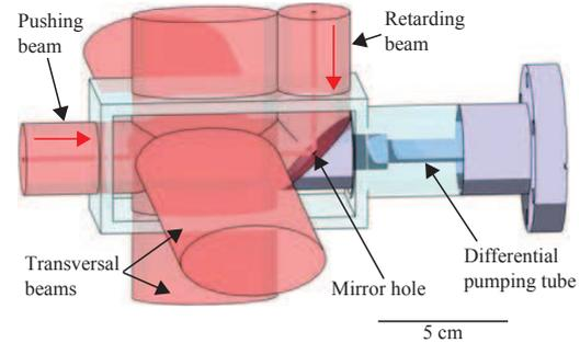
**Fig. 7.** (Color online) Sketch of the parallelepipedical glass cell used for the  $^{40}\text{K}$  2D-MOT. A mirror is placed inside the vacuum chamber to allow an independent control over the longitudinal beam pair. The mirror has a hole in its center and creates a dark cylindrical region in the reflected beams.
