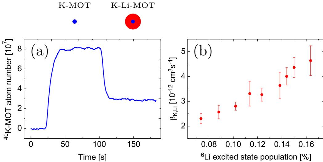
Figure 3.12: (a) Evolution of the atom number in the  $^{40}\text{K}$ -MOT in the absence ( $t < 100$  s) and presence ( $t > 100$  s) of the  $^6\text{Li}$ -MOT for an increased magnetic field gradient of 16 G/cm. (b) Trap loss coefficient  $\beta_{\text{KLi}}$  for heteronuclear collisions as a function of the relative excited-state population of the trapped  $^6\text{Li}$  atoms.
