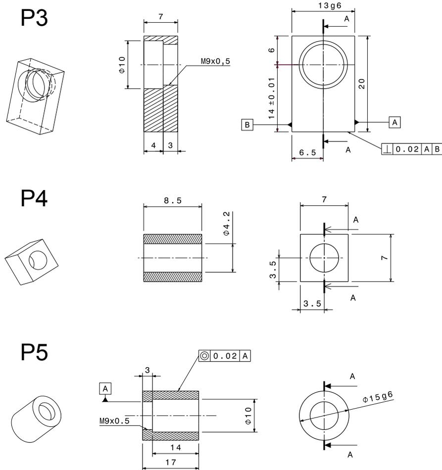
Figure C.5: Engineering drawings of the mounts for the output collimation lens (P3), the isolated blade connectors (P4) and the input collimation lens (P5). Required precision:  $\pm 0.1$  mm, except specified otherwise.
