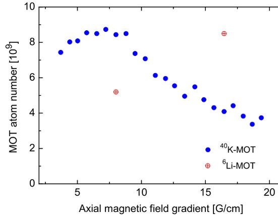
Figure 3.9: MOT atom number as a function of the axial magnetic field gradient. The atom number in the  $^{40}\text{K}$ -MOT is maximum for a gradient of 8 G/cm. This gradient is chosen for the dual-species operation. The  $^6\text{Li}$ -MOT contains more atoms for higher magnetic fields.
