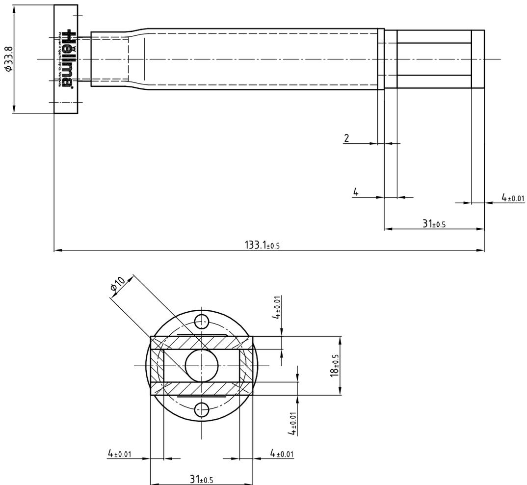
Figure C.1: Engineering drawings of the vacuum science cell (from Hellma GmbH). Indicated dimensions are in units of mm. Additional specifications are given in Sec. 2.2.1.
