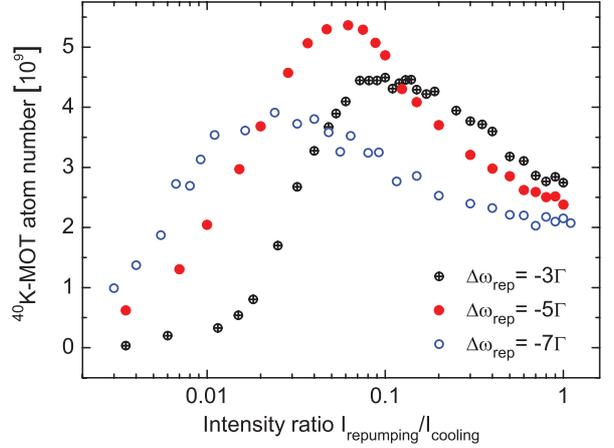
**Fig. 13.** (Color online)  ${}^{40}\text{K}$ -MOT atom number as a function of the intensity ratio between repumping and cooling light for three different repumping detunings  $\Delta\omega_{\text{rep}}$  and a constant cooling light power of 18 mW per MOT beam (which corresponds to an intensity of  $6 I_{\text{sat}}$ ).
