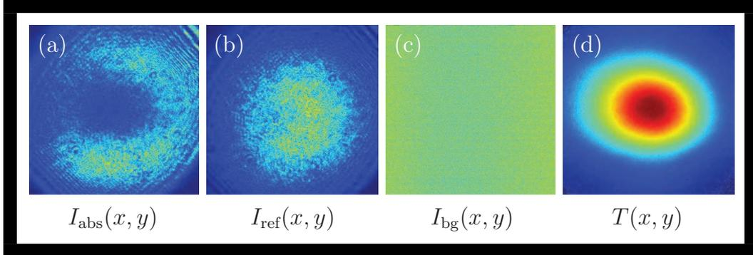
Figure 2.14: Obtaining a normalized transmission profile  $T(x, y)$  requires to take three images: (a) an image of the probe beam after passing through the atom cloud, (b) an image of the probe beam in absence of the atoms and (c) a background image. These are processed according to Eq. (2.6) to give the normalized transmission image (d). The picture shows a magnetically trapped cloud of  $\sim 3 \times 10^9$   $^{40}\text{K}$  atoms.
