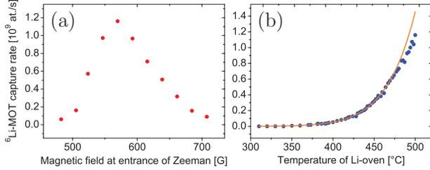
**Fig. 6.** (Color online)  ${}^6\text{Li}$ -MOT capture rate as a function of (a) the axial magnetic field of the Zeeman slower and (b) the temperature of the Li-oven. Circles represent the experimental data and the solid curve the theoretical prediction from equation (3).
