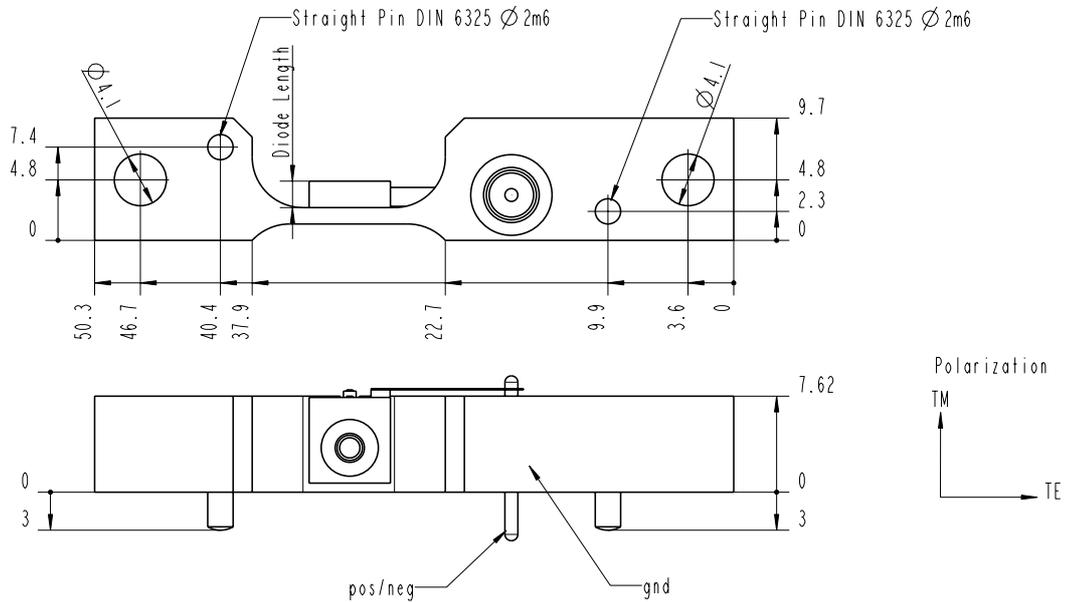
Figure C.7: Engineering drawings of the tapered amplifier chip for lithium (Toptica, ref. TA-670-0500-5), to be mounted on the homemade support whose design is detailed in the subsequent figures.
