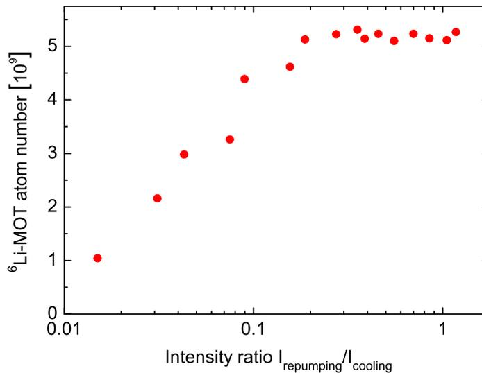
Figure 3.11:  ${}^6\text{Li}$ -MOT atom number as a function of the intensity ratio between repumping and cooling light for a constant cooling light power of 11 mW per MOT beam (which corresponds to an intensity of  $2I_{\text{sat}}$ ). In comparison to  ${}^{40}\text{K}$  (Fig. 3.10 (a)), the optimum atom number requires a larger intensity in the repumping light, which is a consequence of the unresolved excited hyperfine structure of  ${}^6\text{Li}$ .
