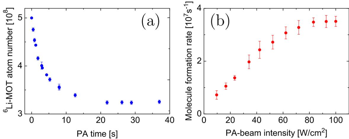
Figure 4.16: (a) Atom number in the  ${}^6\text{Li}$ -MOT as a function of the exposure time of the resonant PA light for the resonance  $\Omega = 1^{\text{up}}, v = 2, J = 1$  at a PA detuning of  $-14.4 \text{ GHz}$  with a PA beam intensity of  $100 \text{ W}/\text{cm}^2$ . (b)  ${}^6\text{Li}{}^{40}\text{K}^*$  molecule formation rate as a function of the PA beam intensity for the same molecular transition.
