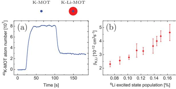
**Fig. 16.** (Color online) (a) Evolution of the atom number in the  ${}^{40}\text{K}$ -MOT in the absence ( $t < 100$  s) and presence ( $t > 100$  s) of the  ${}^6\text{Li}$ -MOT for an increased magnetic field gradient of 16 G/cm. (b) Trap loss coefficient  $\beta_{\text{KLi}}$  for heteronuclear collisions as a function of the relative excited state population of the trapped  ${}^6\text{Li}$  atoms.
