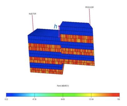
Figure 3.8: IC Fault Model
