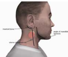
Figure 1: Position of NAM microphone.
