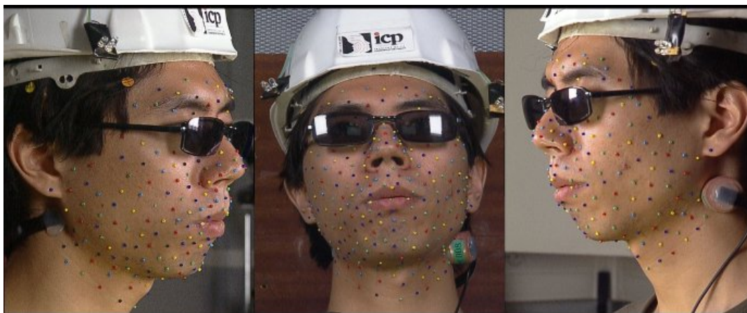
Figure 3.4. Three views of the apparatus used to record the audiovisual data. Colored beads are glued on the speaker's face, to capture facial movements. The NAM microphones are strapped to the speaker's neck. The speaker wears a helmet to restrain head movements.
