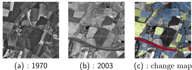
FIGURE 6.3 – Change detection (a–b) : input images ; (c) : the change detection. Yellow : change of cultures ; Blue : abrupt changes ; Red : new roads.
