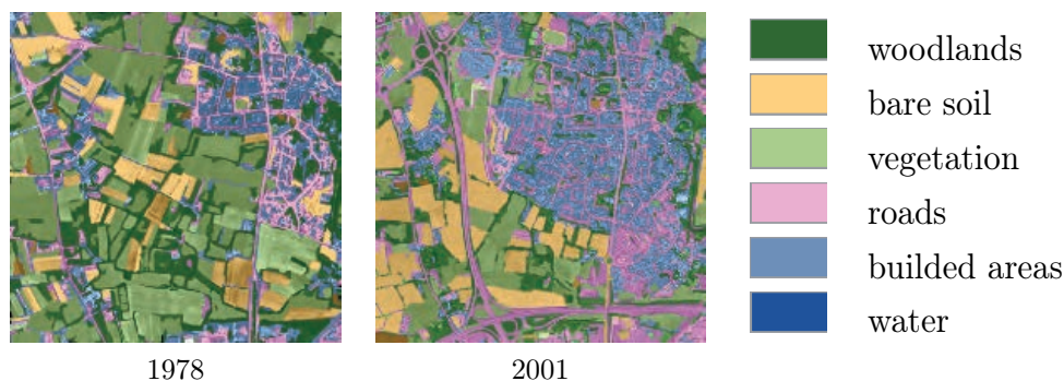
FIGURE 5.5 – Supervised segmentation Two VHSR images from 1978 and 2001, the associated segmentation and the legend.
