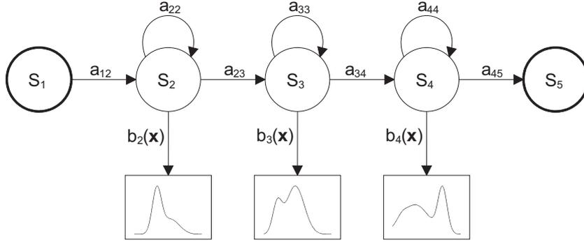
Figure 2.1 — A left-to-right sample HMM diagram.
