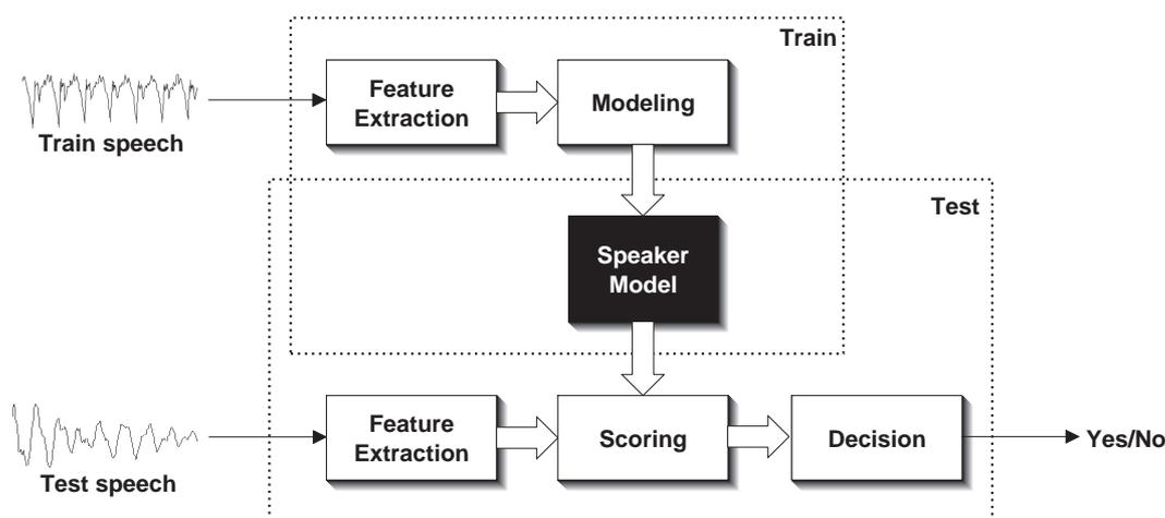
Figure 1.1 — Block diagram of a generic ASV system.
