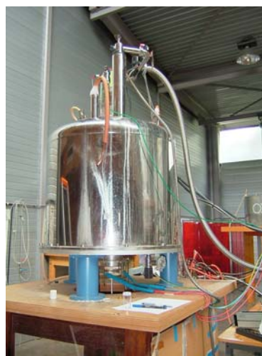
Figure 2-2: High-temperature Faraday Balance with Oxford superconducting coil in the CNRS/CRETA laboratory.
