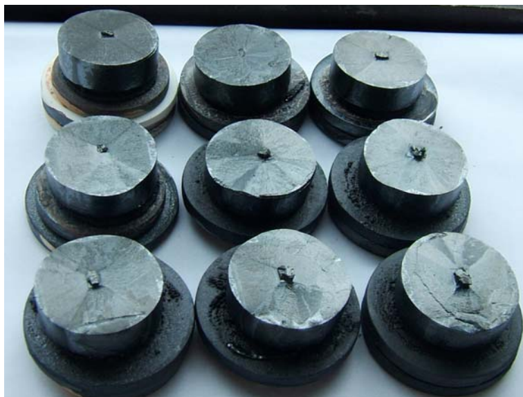
Figure 3-8 Superconductor PMP-YBCO single domain with \Phi 30\text{mm} \times 15\text{mm} size prepared in one batch.
