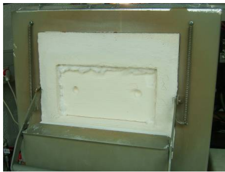
Figure 3-19 Muffle furnace M1 with the door closed keeping primary air atmosphere.
