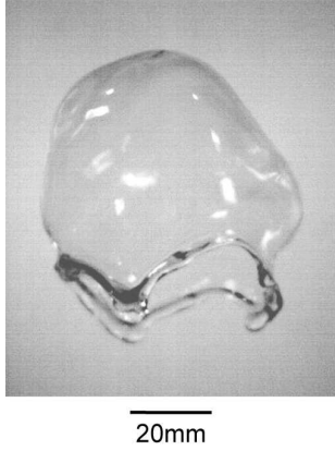
Fig. 3: Transient shape of a very large falling water drop (of initial diameter D_o = 1.8 \pm 0.2 cm, and falling velocity V = 6.2 \pm 0.6 m/s). The drop is a bag, consisting of a water shell surrounding air and bounded at the bottom by a rim. The bag quickly inflates as a function of time (fig. 4), allowing it to expand by a factor of order 3 (that is, 30 for the volume), before bursting.
