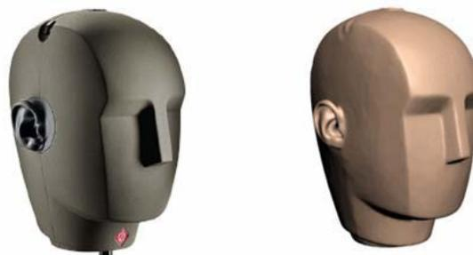
Figure 3 Real Neumann KU-100 dummy head and reference mesh model.
