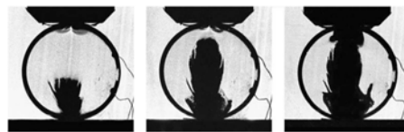
(b) Glass discs failure at 46kN.
