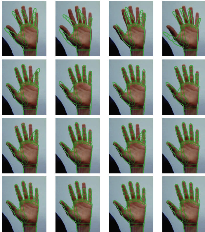
Descriptio 3.25: Each raw corresponds respectively to 1) the initial pose 2) the optimal pose found with the Matlab®function fmincon (BFGS-SQP) after 90 iteration 2) the optimal pose found with the variable-metric method after 90 iterations 3) the optimal pose found with the trust-region method after 90 iterations.
