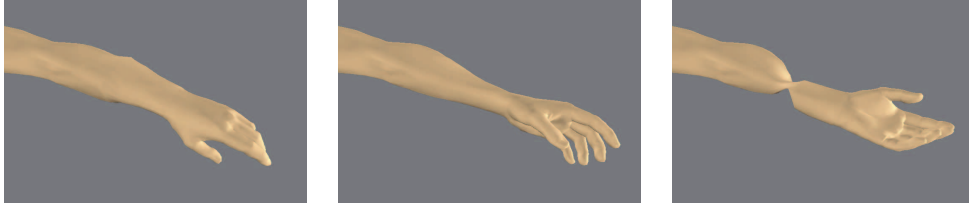
Descriptio 4.2: candy-wrapper artifact when the forearm rotates with an the angle \pi
