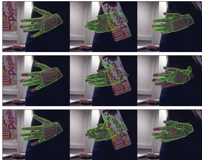
Descriptio 3.31: Tracking results comparisons: each row corresponds respectively to the smart particle filter, the classical particle filter and the single hypothesis method
