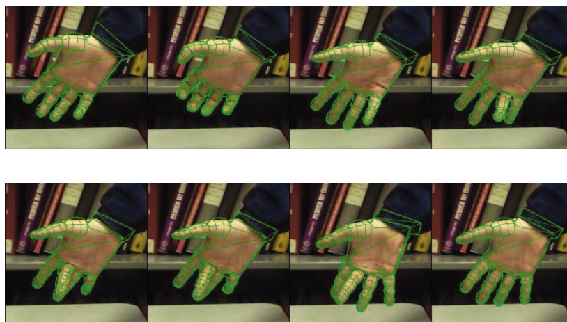
Descriptio 3.29: Eight frames from a tracking sequence provided by authors of [Sudderth 2004] in which the hand makes grasping motions and individual finger movements. The result are qualitatively equivalent
