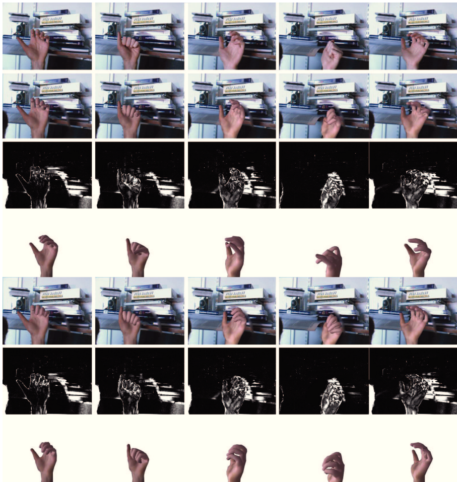
Descriptio 4.18: Second sequence. Each row shows (from top to bottom) (1) the observed image, (2) the final synthetic image with limited pose space, (3) the final residual image, (4) the synthetic side view with an angle of 45^\circ , (5) the final synthetic image with full pose space, (6) the residual image and (7) the synthetic side view
