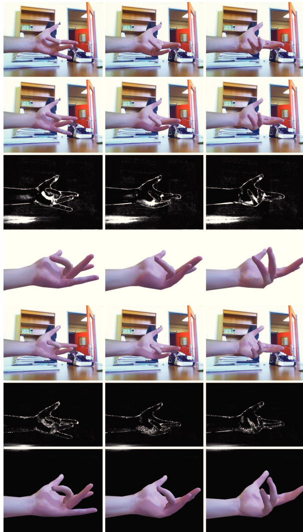
Descriptio 4.16: First sequence illustrating improvement due to self-occlusion forces. The three columns contain results from three separate frames in the sequence. Each row shows (from top to bottom) (1) the observed image, (2) the final synthetic image, (3) the final residual image, (4) a synthetic side view at 45^\circ , (5) the final synthetic image with residual summed on surface, (6) the residual for visible points on the surface, and (7) the synthetic side view
