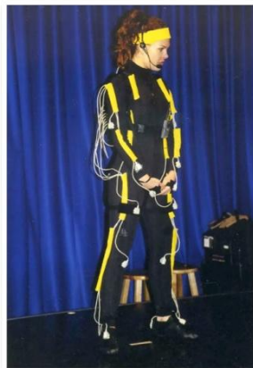
Figure 2-3 : A performer wearing a suit for magnetic motion capture (AMM, 2010)
