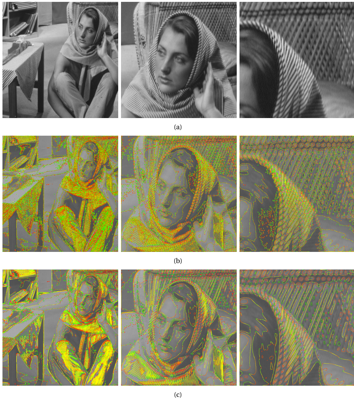
Figure 7.16: Image curvature microscope. (a) the original image, 2X zoom and 4X zoom of the up-right corner; (b) curvature map computed on the original level lines with a quantization step s = 36 ; (c) curvature map computed on shortened level lines at normalized scales l = 1 , l = 2 , and l = 4 (the zoom factor must be equal to the normalized smoothing scale). The left column permits to observe the curvature densities. A zoom is necessary to observe the single curvatures. The middle column and right column focus more and more on shape and texture details.
