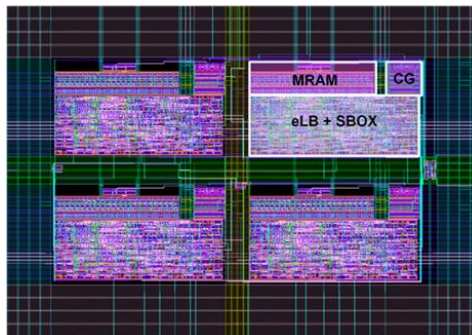
Fig. 5.18: MRAM 130nm small 4 LUT-4 Test Chip (ST CMOS + Crocus MRAM)
