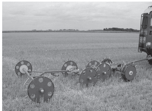
Figure 2-5. MUCEP : MUIlti Continuous Electrical Profiling (Samouëlian et al., 2005).
