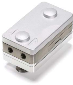
Figure I-7 : Cellule liquide contenant le cristal de quartz
