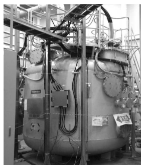
Figure I-9 : Prototype de 10 MW/5.5 kWh, Nikko, Japon.
