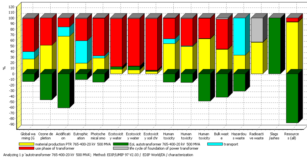
Fig. 3-17 : Characterization result of 765/400/20 kV, 500 MVA power transformer
