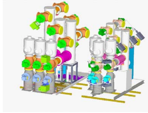
Fig. 1-15 : compact dimensions of the new GIS (right) compared with the former GIS (left)
