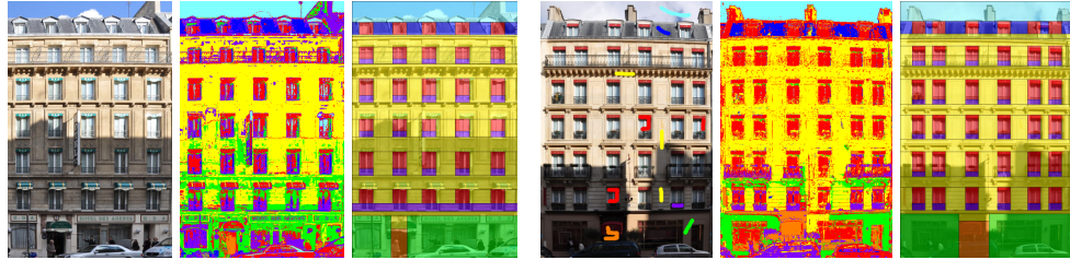
Figure 5.16: Robustness to cast shadows. Huge shadows are cast onto the facades. This is solved by the parsing algorithm both by taking it into account in the data term and treating the misclassified part of the facade as occlusions.
