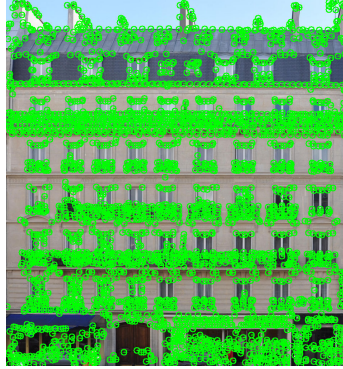
Figure 3.2: Sift descriptors. The orientation is represented by the line inside the circles and the scale is represented by the radius of the scale.
