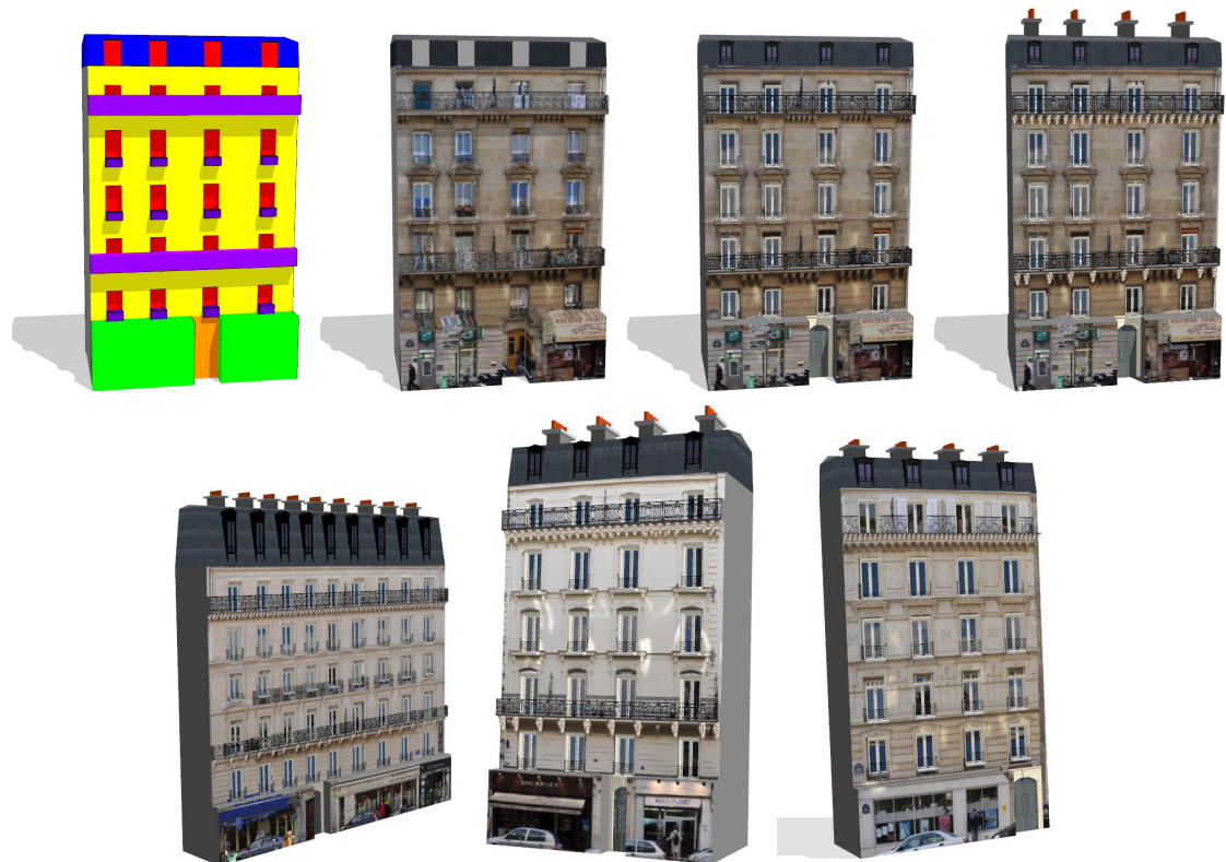
Figure 5.18: From 2D parsing to 3D models. On the first row, we display different level of 3D modeling. From left to right: symbolic model, model textured with the facade image, textured model with complex 3D models for some terminal symbols (windows, door, balconies), enhanced complete 3D model. On the second row, we show some other complete models. Once the facades have been parsed, obtaining these 3D models is costless and straightforward.
