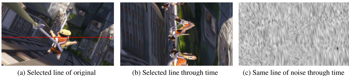
Figure 2.16: Kass and Pesare “coherent noise”. A scan line of the original image (a) is represented over time (from bottom to top) in image (b). Figure (c) displays the evolution of the noise for the same line. The smooth variations of the noise along time and the high correlation with the scene motion illustrate the temporal coherence of this approach. From [KP11].
